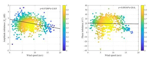
Figure 6. The empirical fitting result of amplitude and phase imbalance relative to wind speed.
