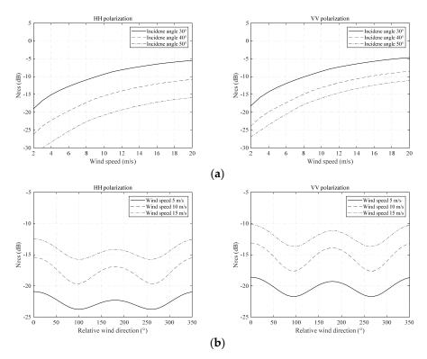
**Figure 7.** (**a**,**b**) The NRCS of sea surface variation relative to wind speed and relative wind direction. Wind speed ranges from 2 m/s to 20 m/s and relative wind direction ranges from  $0^{\circ}$  to  $350^{\circ}$ . Upper row presents NRCS variation at relative wind direction  $0^{\circ}$ , lower row presents NRCS variation at incidence  $40^{\circ}$ .
