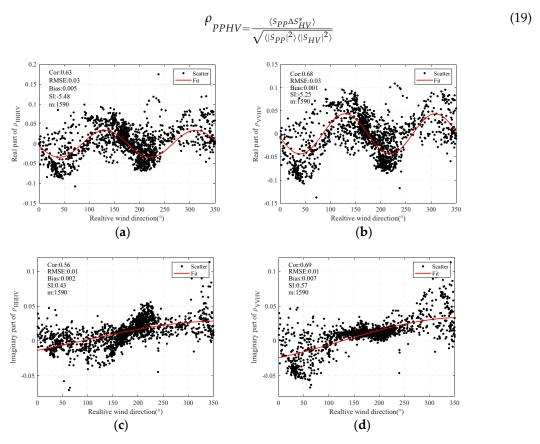
**Figure 13.** Performance of polarization correlation coefficient  $\rho$  variation relative to relative wind direction: (a) Real part of  $\rho_{HHHV}$ ; (b) Real part of  $\rho_{VVHV}$ ; (c) Imaginary part of  $\rho_{HHHV}$ ; (d) Imaginary part of  $\rho_{VVHV}$ .
