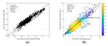
**Figure 12.** Performance of corrected NRCS on wind speed retrieval: (a) NRCS derived from SAR variation relative to CMOD5.N model; (b) The SAR-derived wind speed variation relative to ECMWF wind speed.
