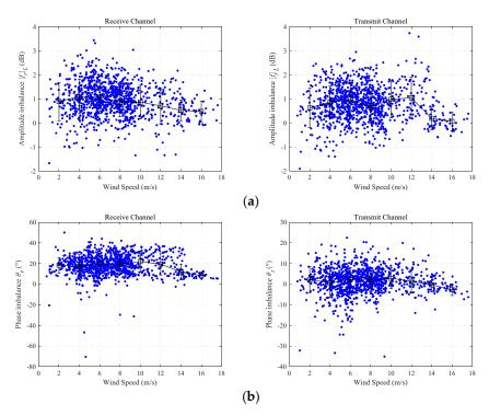
**Figure 4.** (**a**,**b**) The amplitude and phase imbalance of GF-3 SAR imagery of sea surface observation for receive and transmit channel. Upper row represents the amplitude imbalance variation relative to wind speed, and down row represents the phase imbalance variation relative to wind speed.
