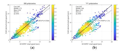
Figure 10. Wind speed retrieval precision for GF-3 SAR HH and VV polarization. The SAR-derived wind speed was compared with on-site wind speed provided by ECMWF: (a) CMOD5.N+PR; (b) CMOD5.N. The color represents the density of scatter points.
