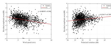
Figure 11. The residual amplitude error variation relative to wind speed and polarization isolation.
