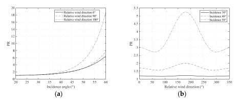
Figure 9. The PR model refitted from GF-3 SAR imagery: (a) Represents the PR variation relative to incidence angle; (b) Represents the PR variation relative to relative wind direction.
