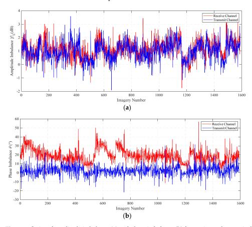
**Figure 3.** Series of amplitude imbalance (**a**) and phase imbalance (**b**) for receive and transmit channel from GF-3 SAR imagery of sea surface observation.
