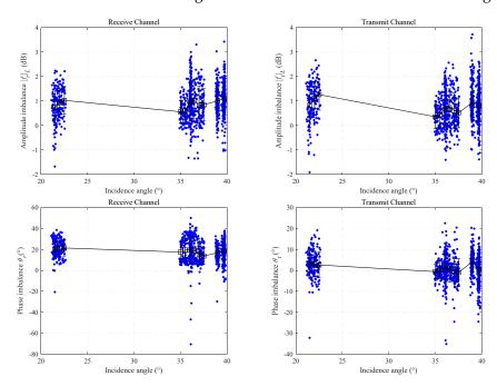
**Figure 5.** The amplitude and phase imbalance variation relative to incidence angle. Same with Figure 4.
