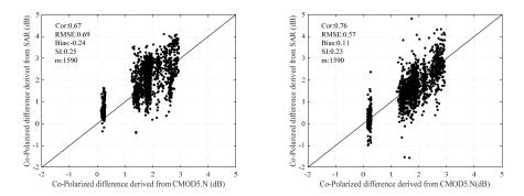
**Figure 8.** The comparison between co-polarization difference from CMOD5.N and GF-3 SAR. Left column presents the original SAR measurement; right column presents the compensated SAR measurement with removal of residual amplitude error.
