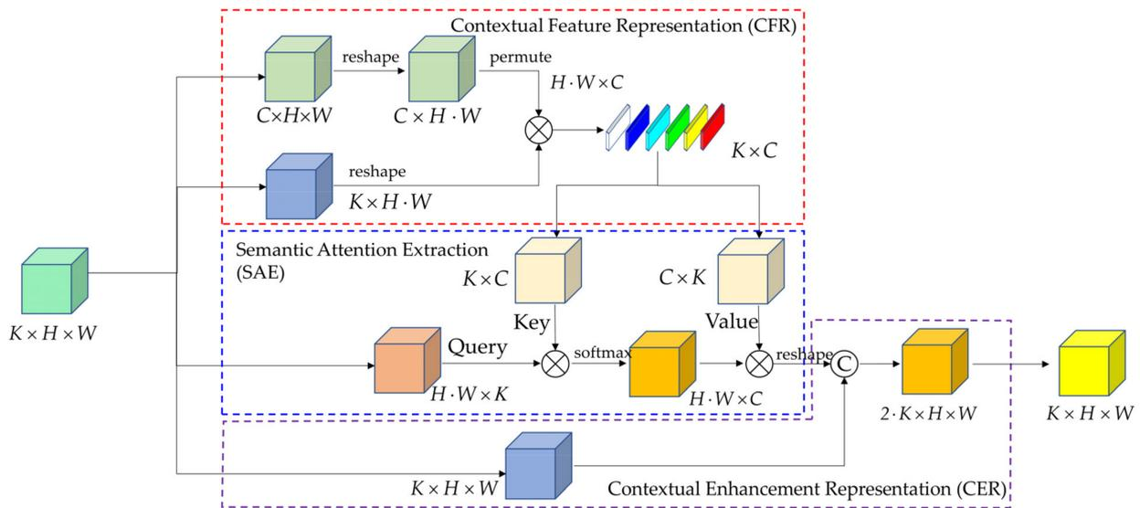
**Figure 3.** The elaborate structure of the context-enhanced module.
