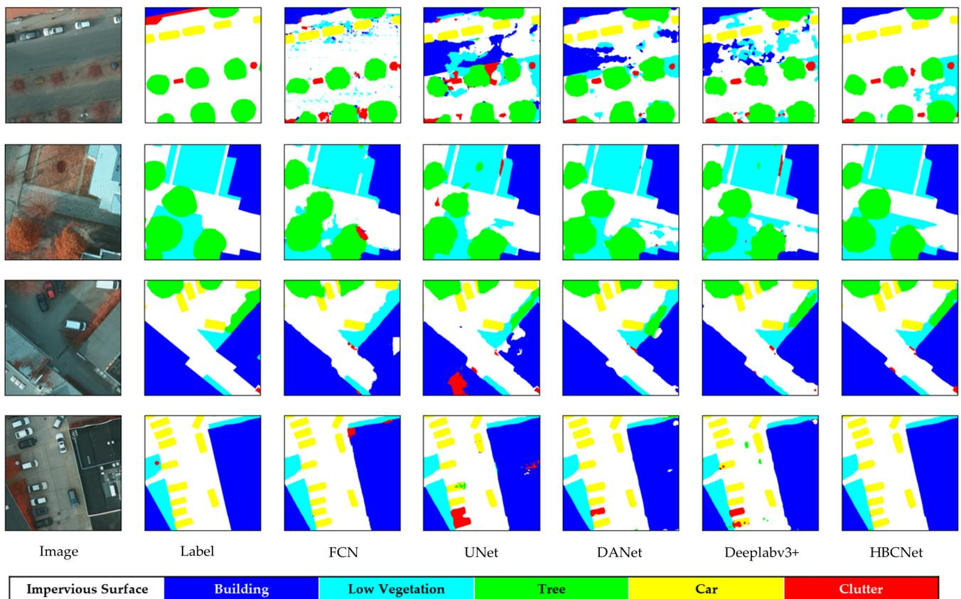
**Figure 7.** Qualitative comparisons between our method and other models for the Potsdam test dataset. (From left to right) Columns demonstrate the original images, the image ground truth, the predictions of FCN, UNet, DANet, Deeplabv3+, and the predictions of HBCNet.
