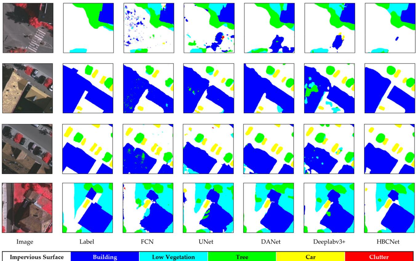
**Figure 6.** Qualitative comparisons between our method and other models for the Vahingen test dataset. (From left to right) Columns demonstrate the original images, the image ground truth, the predictions of FCN, UNet, DANet, Deeplabv3+ and the predictions of our method.
