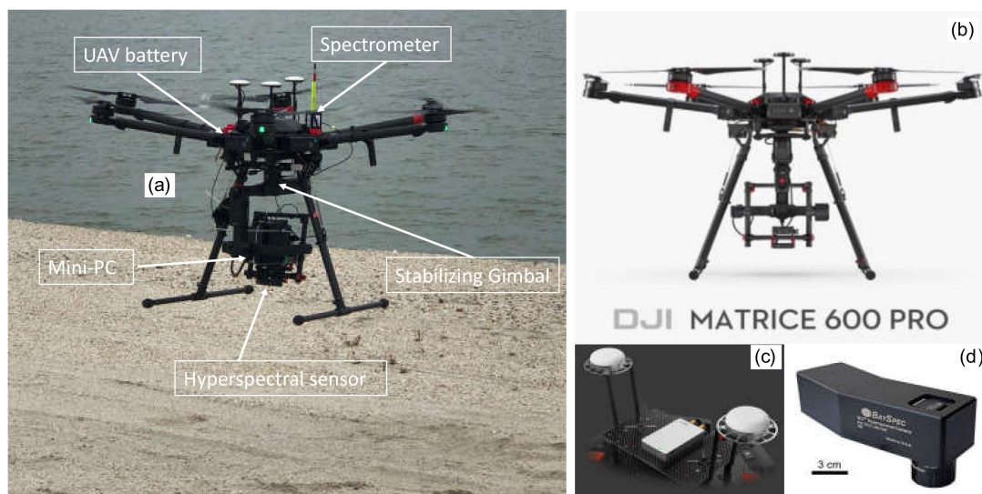
Figure 2. The UAV–airborne imager system (a) that was applied in the study consisted of the DJI Matrice M600 Pro with Ronin MX gimbal (b), a D-RTK GNSS system (c) and a BaySpec OCI-F hyperspectral camera (d) with visible and near-infrared (VNIR) spectrum capabilities.
