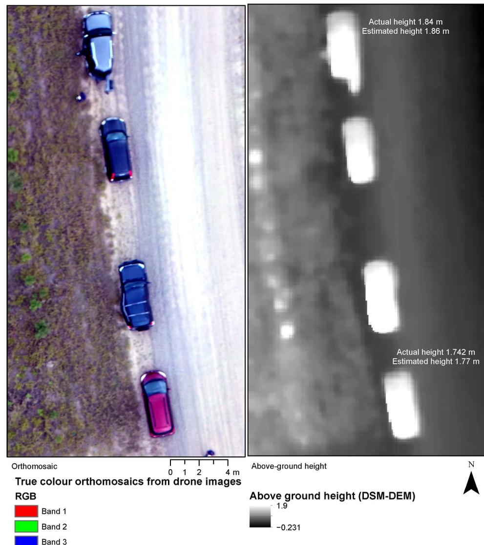
**Figure 3.** Use of parked vehicles with known height to check above-ground height estimated from drone-derived data.
