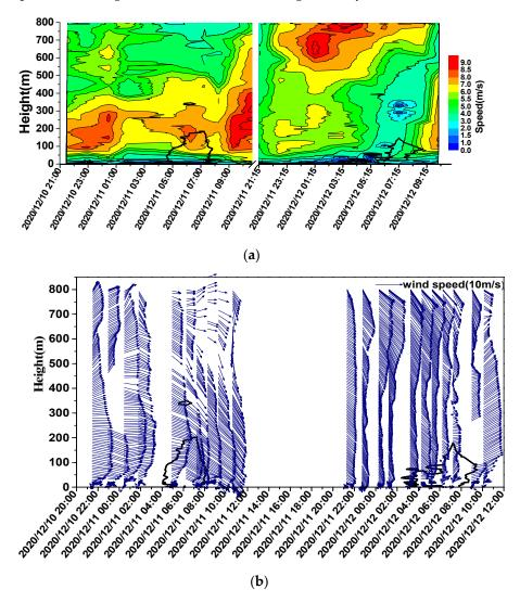
**Figure 5.** (a) The vertical structure of wind speed and (b) The temporal variation in the horizontal wind field (observation by UAV) during the fog–haze process from 10 to 12 December 2020 in Donghai of Lianyungang, China (unit: m/s). Black line: the height of the fog layer.
