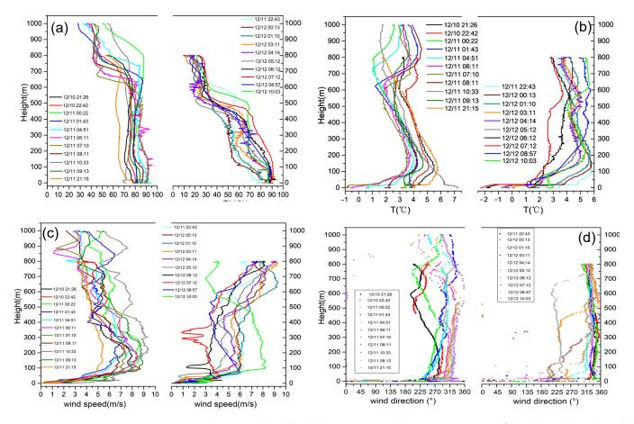
**Figure 6.** The vertical profile of (**a**) RH (unit: %), (**b**) Air temperature (°C), (**c**) Wind speed (m/s) and (**d**) Wind direction (°) during the fog–haze process from 10 to 12 December 2020 in Donghai of Lianyungang, China.
