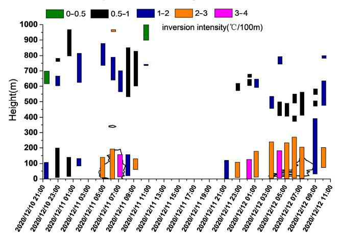
**Figure 7.** The evolutions of inversion layers and inversion intensity during the fog-haze process from 10 to 12 December 2020 in Donghai of Lianyungang, China. Bottom bar: Inversion bottom; top bar: inversion top; inversion intensity:  $^{\circ}C/100$  m. Black line: the height of the fog layer.
