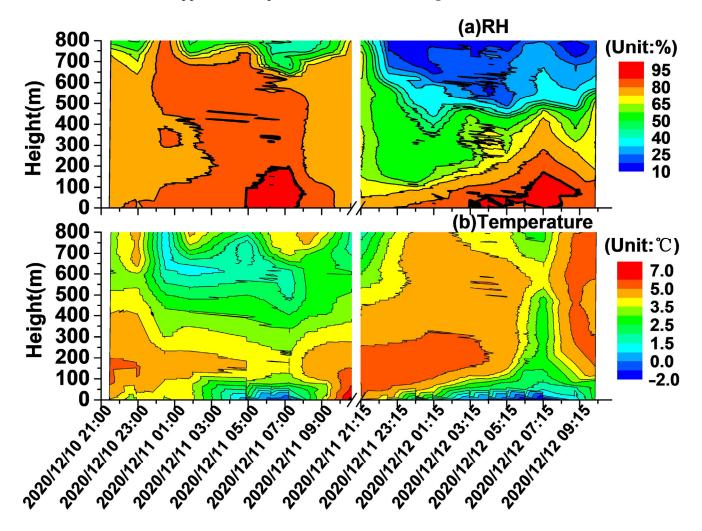
**Figure 4.** (a) RH (unit: %) and (b) Temperature (unit: °C) (observation by UAV) of the vertical structure evolution during the fog-haze process from 10 to 12 December 2020 in Donghai of Lianyungang, China.
