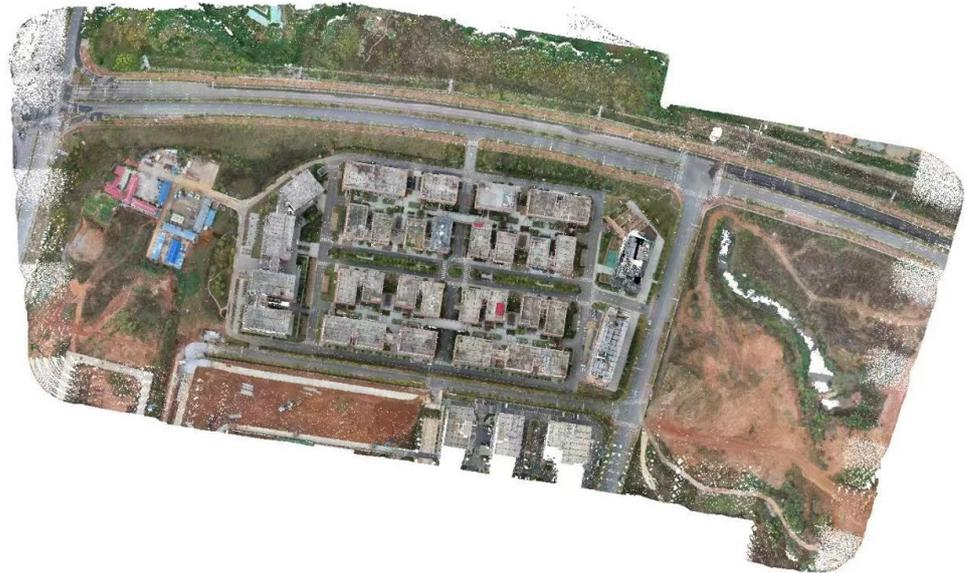
**Figure 3. The map of AirLoc.** The geometric structure of AirLoc is provided by Airborne LiDAR, which allows the quick measurement of distance between LiDAR sensor and the surface of objects it scans, accurately mapping 3D models of outdoor area.
