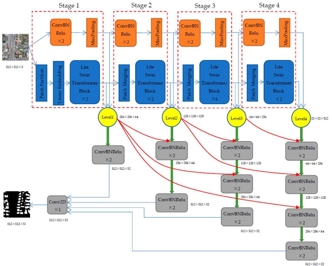
**Figure 1.** Architecture of the LiteST-Net network model. The orange part is the convolution module, the blue part is the Lite Swin transformer module, and the yellow part shows the extracted features of different levels. The gray part is the decoding module, in which the thick green down arrow is the transpose convolution, and the red curve is the addition of features. The number in the lower right corner of blocks shows the size and channels of the feature.
