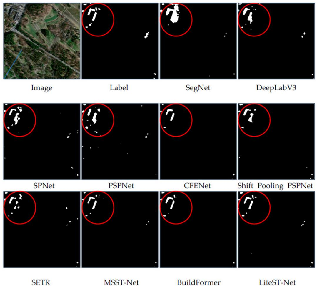
**Figure 7.** Prediction of small buildings on the Massachusetts building test dataset. The red circle shows the predicted results of various models for the same small building.
