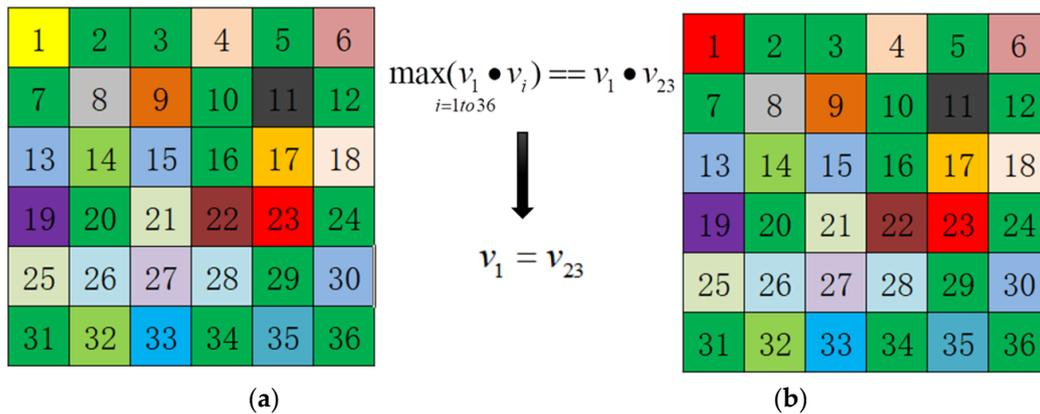
Figure 3. Schematic diagram of maximum weight replacement of the Lite Swin transformer. The number is the sequence number of the pixel, and the color is the feature value of the pixel, that is,  $v$  in Lite Swin transformer. (a) is the feature map before the Lite Swin transformer, and (b) is the feature map of the first pixel after being calculated by the Lite Swin transformer.
