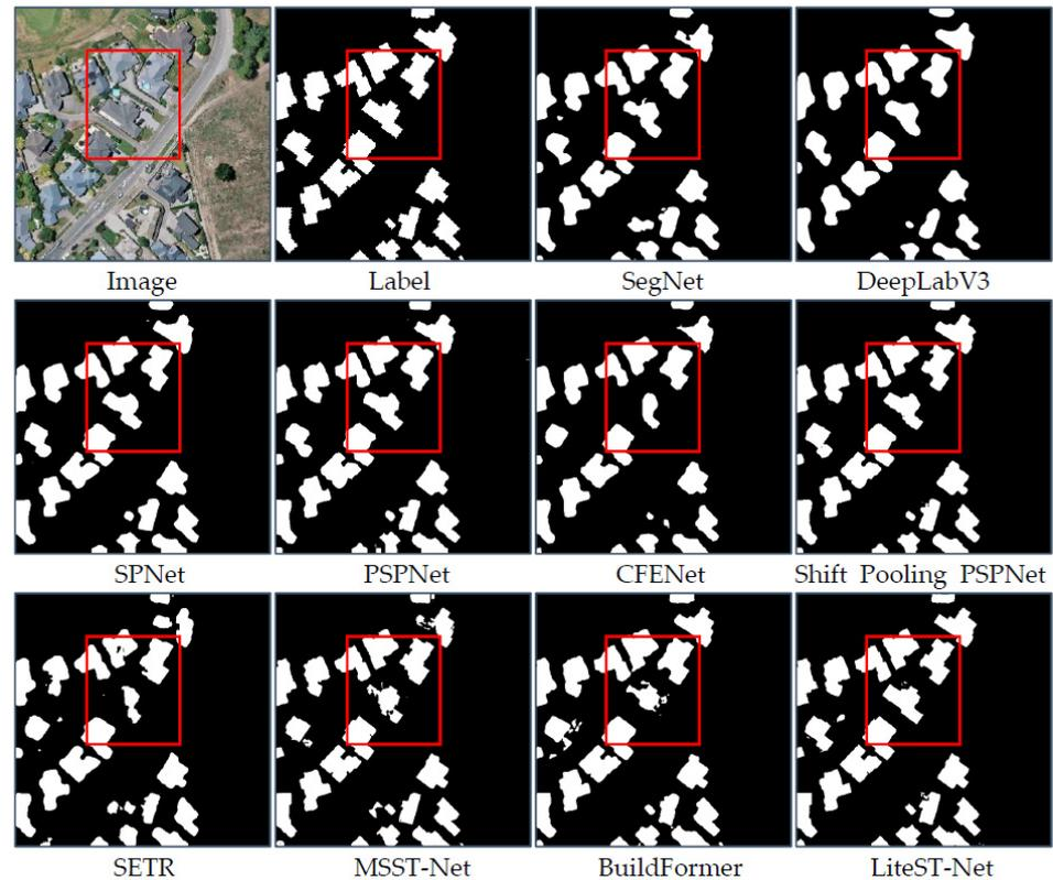
**Figure 4.** Prediction of classic networks for small buildings on the WHU building test dataset. The red box shows the predicted results of various models for the same small building.
