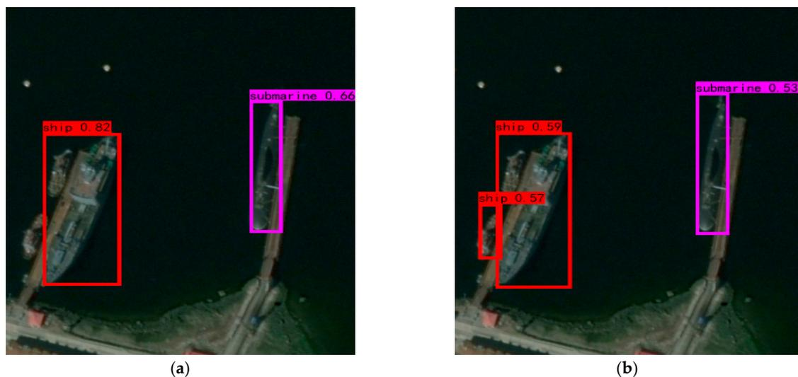
**Figure 6.** Comparison of detection performance between the original and improved algorithms: (a)YOLOX detection result, (b) E2YOLOX-VFL detection result.
