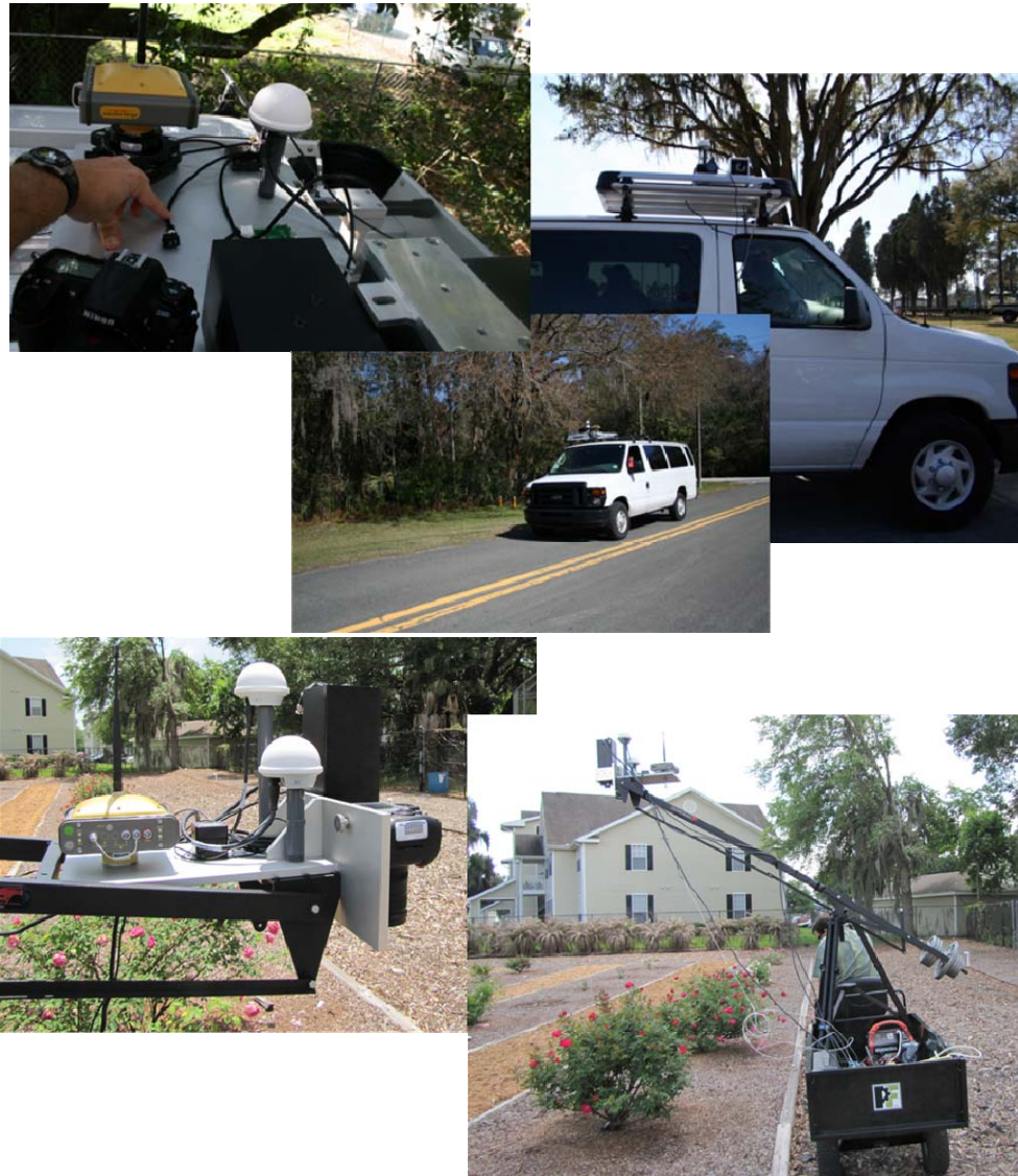
Figure 5. Imaging system mounted on a van (top) and on a boom carried by a tractor trailer (bottom).
