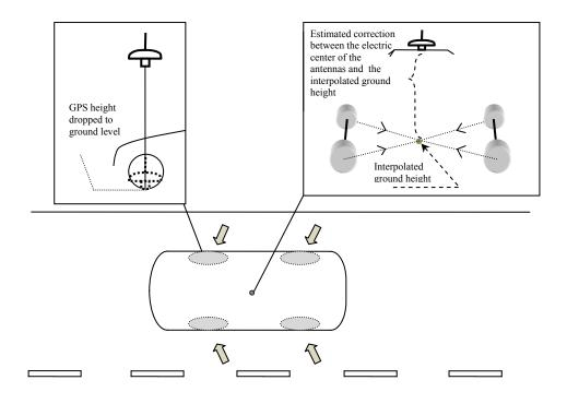
If the vehicle is not level during data acquisition, a small error is generated, due to the drop in the GPS observation directly downwards relative to the GPS height calibration. In these cases, the angle of the vehicle should be taken into account when determining the corrected heights. However, the road slopes in our test area were not steep enough to require this kind of correction.
