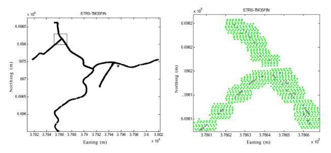
During GPS data acquisition, measurements were collected using the "fixed" mode. In the "fixed" mode, the GPS delivers centimeter-level positioning precision if the integer estimate of the ambiguity search succeeds. The speed of the vehicle was maintained at approximately 30 km/h to achieve the desired point density. When the receiver dropped out of "fixed" mode, the vehicle was stopped until
