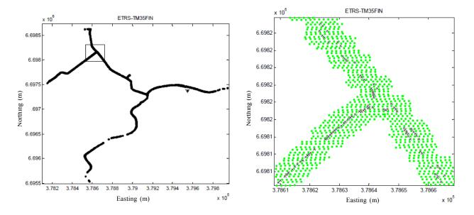
**Figure 4.** Real-time kinematic (RTK) GPS observations along the test area roads. Left: The complete test area. The RTK reference station is marked with a triangle. Right: A detailed view from the test area; the location of the detailed view is marked with a square in the left image. GPS observations are illustrated with black crosses, and ALS points near GPS observations are represented by green dots.
