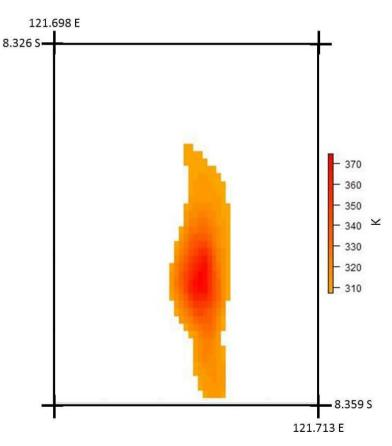
The total radiant flux density associated with the thermally anomalous pixels isolated (Q in W), and that associated with the values of  $\overline{bg_{10}}$  (*i.e.*,  $Qbg_{10}$ ), was then calculated using the Stefan Boltzman equation (Equation (1)) incorporating both the pixel brightness temperature (T in K) and area (A, 10,000 m<sup>2</sup>):
