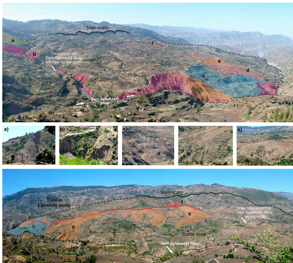
Figure 2. Panoramic view of the Debre Sina landslide from the SE (above) and E (below) with examples of characteristic geodynamic features within the main landslide body and its close surroundings: rockfalls (a); gully erosion along the Dem Aytemashi River and its tributaries (b); rotational landslides (c); debris flows (d); shallow landslide and earthflow (e); and displaced rock blocks with well-marked scarp lines (f). The estimated position of the shear plane outcrop is shown as a blue line. All photos were taken in March 2015 by Zuzana Vařilová.
