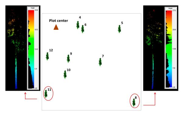
Figure 11. Reduction of the laser pulse penetration due to tree shadowing.
