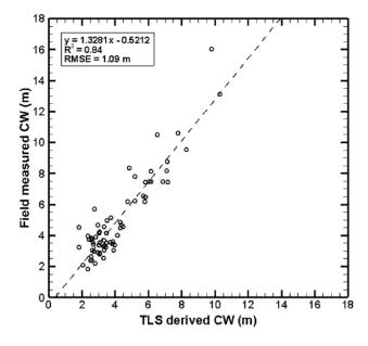
**Figure 10.** Scatterplot of regression result for field measured crown width and terrestrial laser scanning (TLS) derived crown width.
