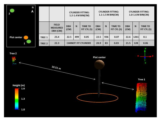
Figure 7. Cylinder fitting results on 1.2–1.4 m height bin for tree 1 and tree 2.
