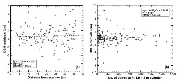
Figure 8. Diameter at breast height (DBH) residuals as a function of (a) distance from scanner (b) number of points to fit the cylinder.
