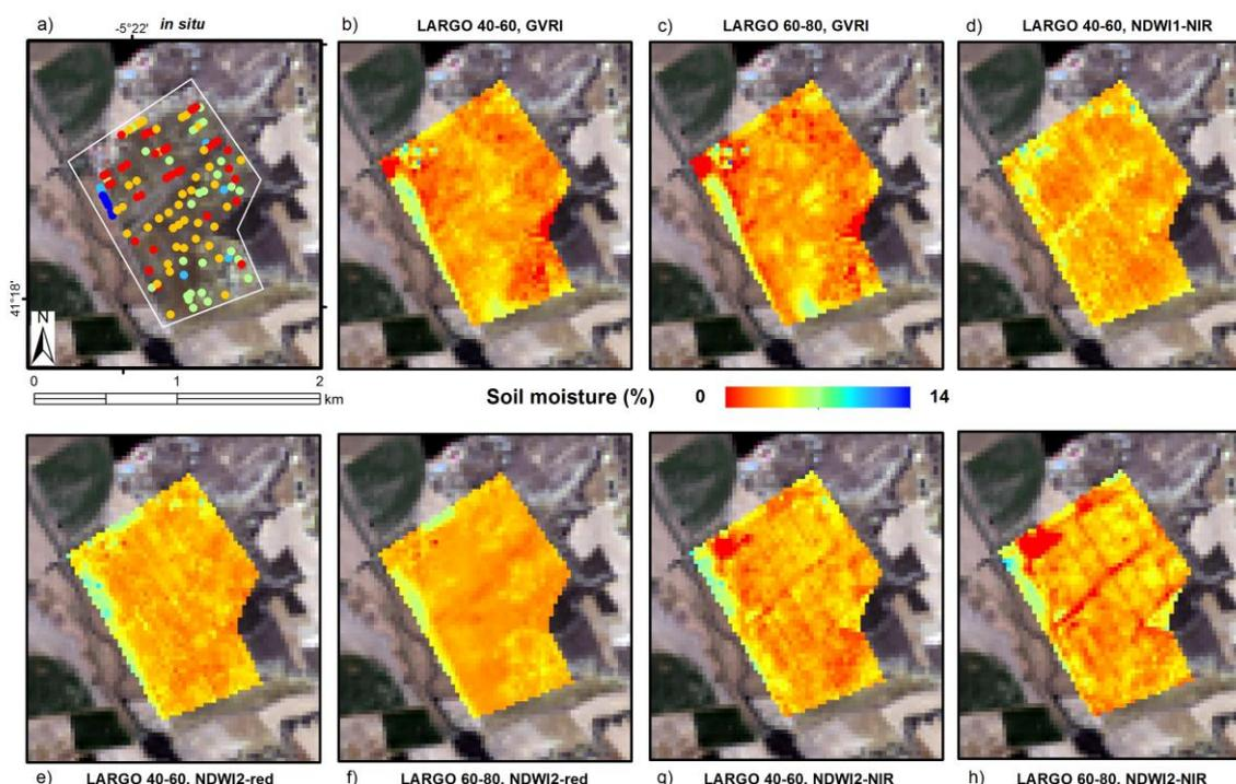
**Figure 7.** (a) Ground observations distribution. (b to h) Estimated soil moisture (% vol.) maps following the seven alternatives considered.
