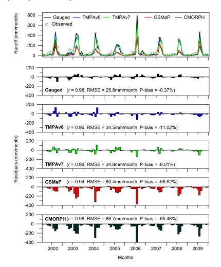
**Figure 6.** Comparison of monthly dam inflow observations and simulations from use of the satellite-derived precipitation products (**top panel**) and the respective residuals (**lower panels**) calculated as the monthly observation minus the simulated value.
