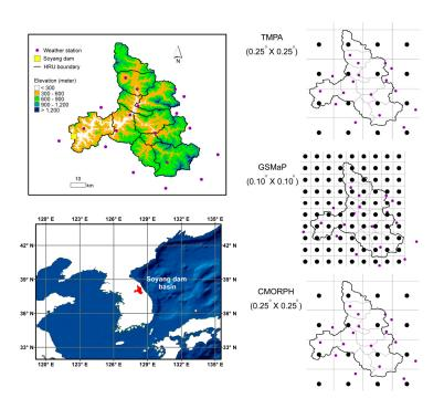
**Figure 1.** Location, elevation, and hydrologic response unit (HRU) boundaries of the Soyang dam basin with locations of the 19 weather stations displayed on the left. The spatial resolution of the tropical rainfall measuring mission (TRMM) multi-satellite precipitation analysis (TMPA), global satellite mapping of precipitation (GSMaP), and climate prediction center (CPC) morphing technique (CMORPH) precipitation products over the Soyang dam basin are displayed on the right.
