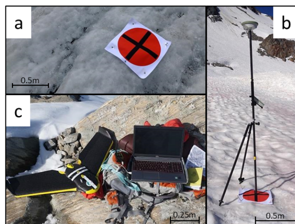
Figure 2. Example of a GCP set on (a) ice and (b) snow. The GCP center is measured with a Leica GPS 1200 (b). (c) SenseFly eBee (left) and computer (right) linked to the transmitter sending the flight coordinates to the UAV.
