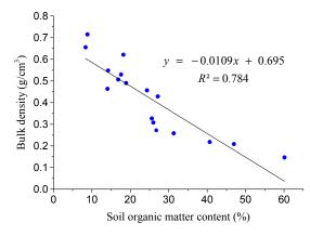
**Figure 2.** Soil organic matter content (*SOM*) and bulk density  $(g/cm^3)$  of the soil samples from the 17 EC-5 *SM* sensor-sites.
