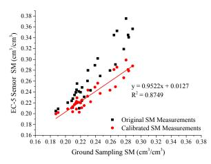
Figure 3. The calibration results of EC-5 SM sensor.
