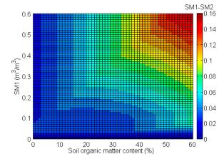
**Figure 8.** The differences between the *SM* values derived by Liu's model (SM1) and the Mironov model (SM2). SM1 ranged from 0 to 0.6 cm<sup>3</sup>/cm<sup>3</sup>, while *SOM* ranged from 0 to 60%. SM1 and *SOM* were input into Liu's model, and SM2 was then retrieved by the Mironov model based on the  $T_B$  that was simulated by Liu's model. The soil was assumed to be bare and smooth.
