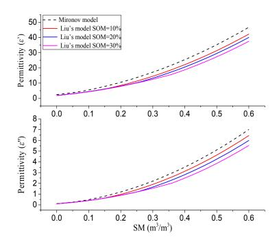
**Figure 5.** Comparison between the dielectric constants simulated by the Mironov model and that simulated by Liu's model for three kinds of soil with the same clay content (13%) and different *SOM* (10%, 20% and 30%) at 1.4 GHz.
