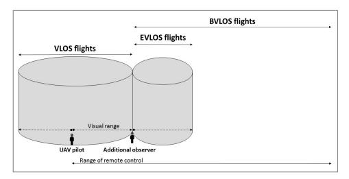
**Figure 5.** Schematic distinction between UAV flight ranges—visual line-of-sight (VLOS), extended visual line-of-sight (EVLOS) and beyond visual line-of-sight (BVLOS), based on [87].
