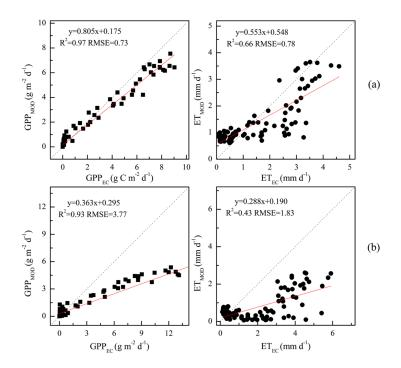
**Figure 7.** The scatterplots of eight-day average GPP and ET between flux tower measurements and MODIS products at the two flux sites during 2013 and 2014. (**a**,**b**) represent the Arou grassland site and the Daman cropland site, respectively. 92 periods of data are used in total. The black dashed line and red line represent 1:1 line and linear fit, respectively.
