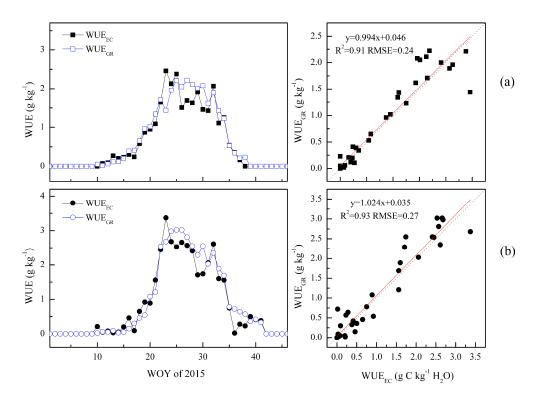
**Figure 5.** Seasonal patterns and the scatter plots of ecosystem water use efficiency between flux tower measurements ( $WUE_{EC}$ ) and the MODIS estimates ( $WUE_{GR}$ ) from time-series EVI data at the two flux sites in 2015. (**a**,**b**) represent the Arou grassland site and the Daman cropland site, respectively. The black dashed line and red line represent 1:1 line and linear fit, respectively.
