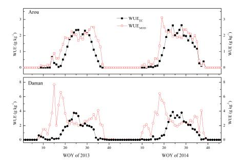
**Figure 4.** A comparison of seasonal variations of ecosystem water use efficiency from flux tower measurements ( $WUE_{EC}$ ) and the estimates from MODIS products ( $WUE_{MOD}$ ) at the two flux sites Arou and Daman during the period of 2013 and 2014.
