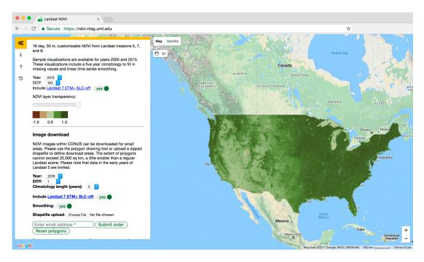
**Figure 5.** A screen shot of the NDVI web application (https://ndvi.ntsg.umt.edu). To download a composite, users set their desired parameters in the left panel. The region of interest can either be an uploaded shapefile or a polygon drawn directly on the map. The composite is processed on the fly and users are notified via email when it is ready to download.
