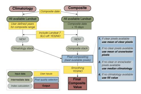
**Figure 4.** A flow chart demonstrating the NDVI compositing process, in which the best available pixels from all available Landsat sensors are selected and combined to produce the final NDVI composite value.
