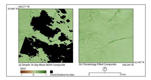
**Figure 2.** (a) A simple 16-day mean NDVI composite from 28 July to 12 August 2015 created from Landsat 7 and 8 sensors. The composite contains missing data due to cloud cover and scene edges are apparent due to differing acquisition dates. (b) A 16-day climatology (5-year) gap filled composite for the same time and location. The climatology is user defined in order to produce an appropriate composite for the question being asked.
