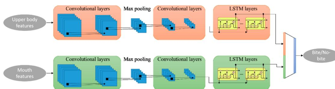
**Figure 4.** Schematic representation of the RABiD algorithm, for the parallel analysis of upper body (including the head) and mouth movements in videotaped meals. The outcome of the algorithm is a complete behavioral description of a single meal including meal duration, total number of meal bites, as well as time series of bite instances across the meal. LSTM: called long short-term memory.
