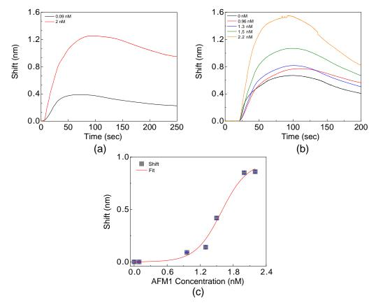
**Figure 5.** Aflatoxin M1 (AFM1) detection in the milk samples. Sensorgrams for concentrated milk samples with different AFM1 concentrations. (a) The first demonstration of AFM1 detection in milk. (b) The second set of tests of AFM1 detection. The black line is the response to the blank eluate. (c) The calibration function for the aMZI based sensor is extracted from the logistic fit of the shift values for different AFM1 concentrations (C).
