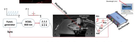
Figure 1. (top left) Image of the chip with illuminated Mach-Zehnder Interferometers (aMZI). (top right) Normalized transmission spectra of four aMZI. (bottom) Schematic of the experimental setup.
