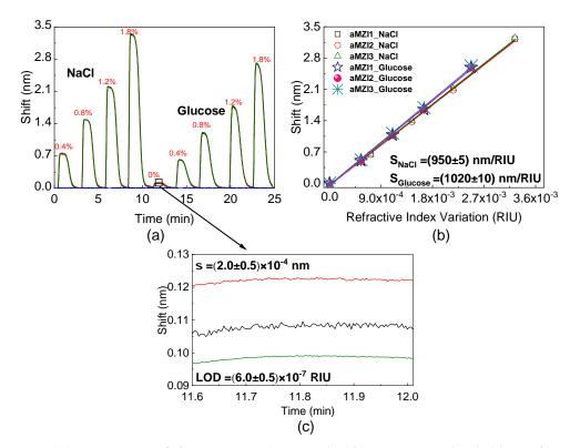
**Figure 3.** (a) Sensorgrams of four aMZI on the same chip for variation in the cladding refractive index, obtained by injections of glucose and salt water solutions at different concentrations (glucose and NaCl concentrations are in  $\frac{w}{v}$ /v labelled on the plot). (b) Wavelength shift linear fit where the slope is the sensitivity. (c) The shift taken in 24 s corresponding to the time interval 11.6 ÷ 12.0 min in the sensorgram. This interval is marked inside the black square.
