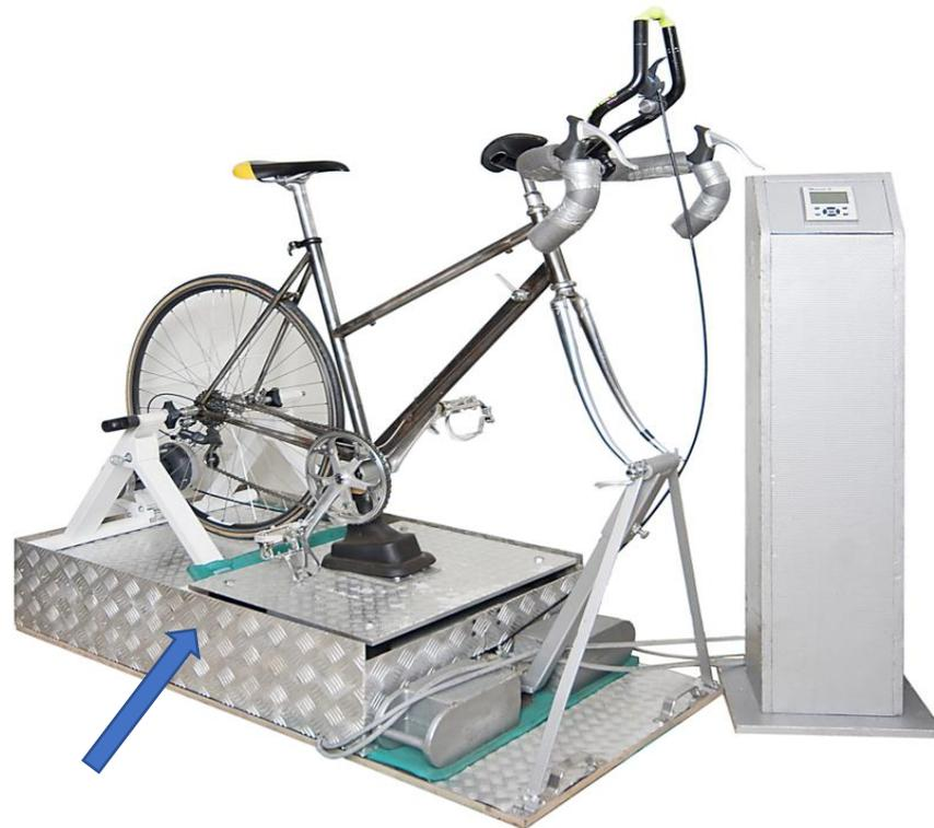
**Figure 1.** The prototype of a vibration ergometer device invented by Dieter Quarz. This photo is presented with his permission. The arrow in the figure shows the vibration platform, which vibrates the bottom bracket and is driven by a strong electromotor with excenter.
