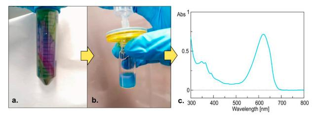
**Figure 7.** (a) Centrifugation of the cellular suspension, (b) filtration, and (c) UV/Vis analysis of the supernatant indicated the presence of phycocyanin in the sample, a typical cyanobacterial pigment.
