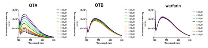
**Figure S6.** Fluorescence spectra (excitation 497 nm) from SG and B08 aptamer and various concentrations of OTA, OTB and warfarin. A concentration dependent decrease in fluorescence occurs with an increasing concentration of OTA; however, very little change in observed upon the addition of OTB and warfarin.
