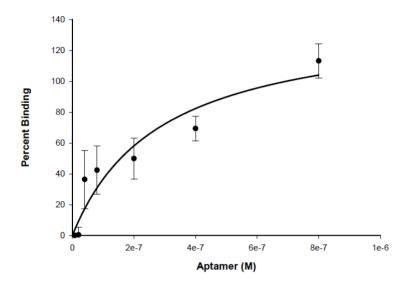
**Figure S4.** Binding isotherm for aptamer B08 with OTA obtained using the magnetic beads-based isocratic elution assay. The curve was generated using Sigma Plot (Version 12.5). The  $K_D$  was determined to be  $110 \pm 50$  nM.
