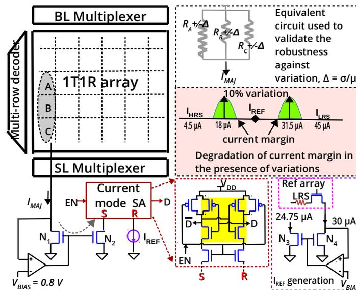
**Figure 5.** Current in the sense path (‘S’) and reference path (‘R’) are compared. ‘D’ and ‘ $\bar{D}$ ’ are precharged to  $V_{DD}$  when  $EN$  is low. When  $EN$  goes high, one of them discharges at a faster rate, which is reinforced by the positive feedback formed by cross-coupled inverters (shaded yellow) [14,15].
