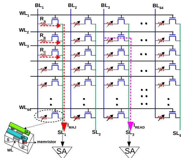
**Figure 4.** In a conventional memory, a single row is activated and  $V_R$  is applied across the cell to read from it (e.g., reading from cell at (2,3) depicted in pink). To compute majority, three Word Lines ( $WL_{1,2,3}$ ) are activated simultaneously and  $V_R/3$  is applied across cells in column 1 resulting in  $I_{MAJ}$ .
