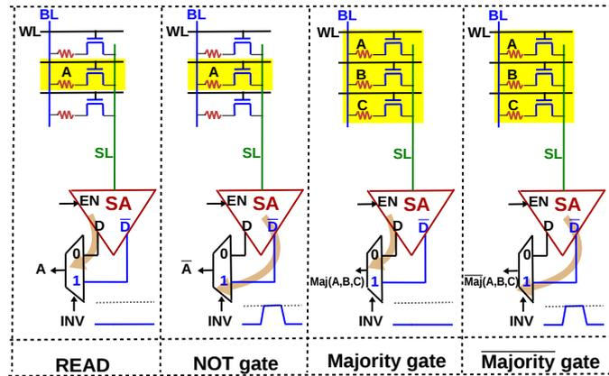
**Figure 8.** With an additional 2:1 Mux at the output of the SA, a NOT gate can be implemented by using the control signal *INV*. Similarly, majority and its complement, *majority* can be implemented. All logic operations are essentially READ operations.
