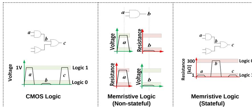
**Figure 3.** In CMOS logic, inputs, outputs and intermediate values are represented as voltages; in memristive logic, inputs, outputs and intermediate values are represented as either voltages or resistances. A memristive logic is said to be stateful if resistance is the only state variable for representing inputs, outputs and intermediate results of computation.
