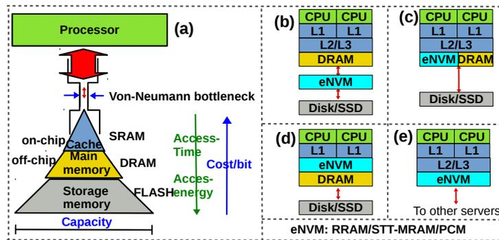
**Figure 1.** (a) The von-Neumann bottleneck. Possible ways in which emerging non-volatile memories (NVMs) (eNVM) can be integrated into the memory hierarchy (b) eNVM can fill the gap between Solid State Drive (SSD) and main memory (c) eNVMs can be integrated alongside main memory (d) eNVMs can be integrated as embedded memory (Last level cache replacement) (e) Universal memory (Main and storage) [1].
