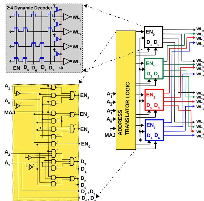
**Figure 7.** Multi-row decoder is implemented by interleaving multiple decoders and using an additional control signal called  $MAJ$ . When  $MAJ$  is logic '0',  $WL_i$  corresponding to row address  $A_3A_2A_1A_0$  is selected. When control signal  $MAJ$  is logic '1',  $WL_i, WL_{i+1}, WL_{i+2}$  are selected.
