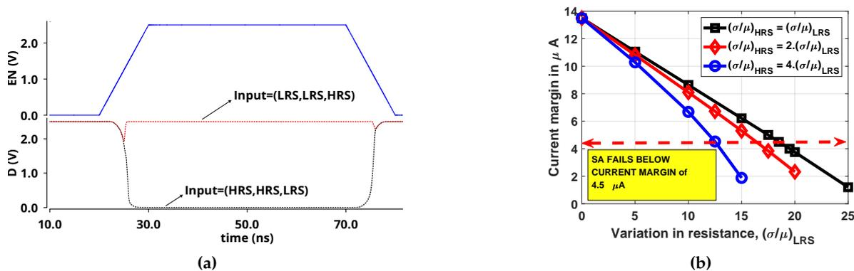
**Figure 6.** (a) A sample output of the Sense Amplifier (SA) for a typical case of sensing with 10% variation in LRS and 40% variation in HRS. EN is the Sense amplifier’s enable signal and, as soon as it goes high, the SA output node (D) is discharged to 0 V (HRS,HRS,LRS) or remains high (LRS,LRS,HRS) (b) Effect of variations in IHP’s cells on current margin.
