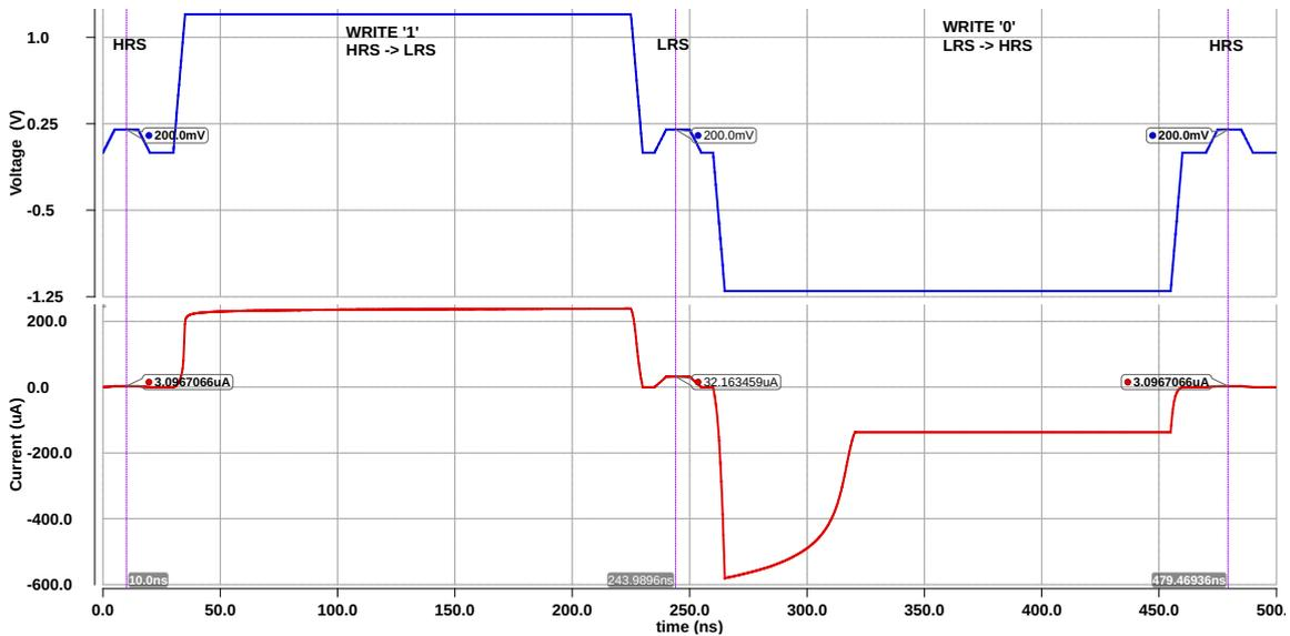
**Figure 9.** Voltage across the RRAM (BL–SL) and the current during WRITE operations. The state of the RRAM cell is detected by a small voltage applied across the cell and measuring the current through it.
