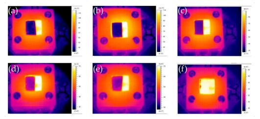
**Figure 5.** The IR thermal images of heat sink surfaces with different treatments at 40 °C: (**a**) without surface treatment; (**b**) chemical polishing; (**c**) chemical coarsening; (**d**) mechanical shot peening; (**e**) chemical oxidation; (**f**) thermal radiation coating.
