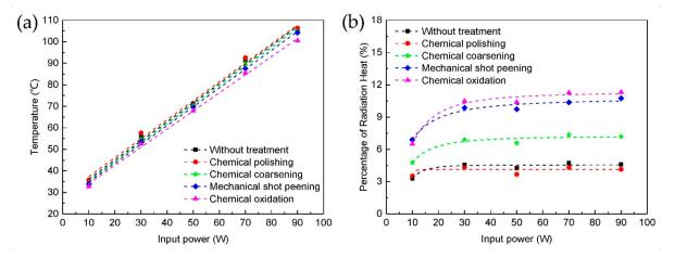
**Figure 6.** Performance of heat sinks with different surface treatment in wind tunnel under different heating power: (**a**) temperature of heat sinks, (**b**) percentage of radiation heat.
