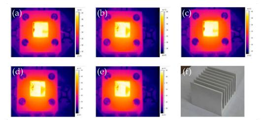
**Figure 8.** The IR thermal images of heat sink surfaces with thermal radiation coating on different treated surfaces: (**a**) without surface treatment; (**b**) chemical polishing; (**c**) chemical coarsening; (**d**) mechanical shot peening; (**e**) chemical oxidation; (**f**) photo of heat sink with thermal radiation coating.
