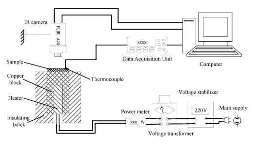
Figure 2. Heat sink surface thermal emissivity test system with infrared (IR) camera.
