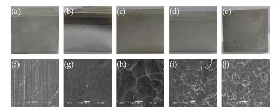
**Figure 4.** Surfaces of heat sinks with different treatment: photos of heat sinks (**a**) without treatment, (**b**) chemical polishing, (**c**) chemical coarsening, (**d**) mechanical shot peening and (**e**) chemical oxidation; SEM images of heat sinks surfaces (**f**) without treatment, (**g**) with chemical polishing, (**h**) chemical coarsening, (**i**) mechanical shot peening and (**j**) chemical oxidation.
