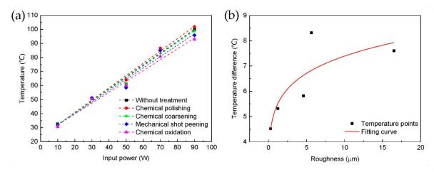
**Figure 9.** Temperatures of heat sinks with thermal radiation coating in wind tunnel: (**a**) influence of different treated surface under the coating; (**b**) temperature difference of heat sinks with and without coating at different surface roughness (heating power 90 W).
