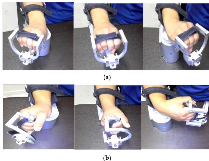
**Figure 3.** (a) Abduction/adduction movement; (b) Flexion/extension movement.
