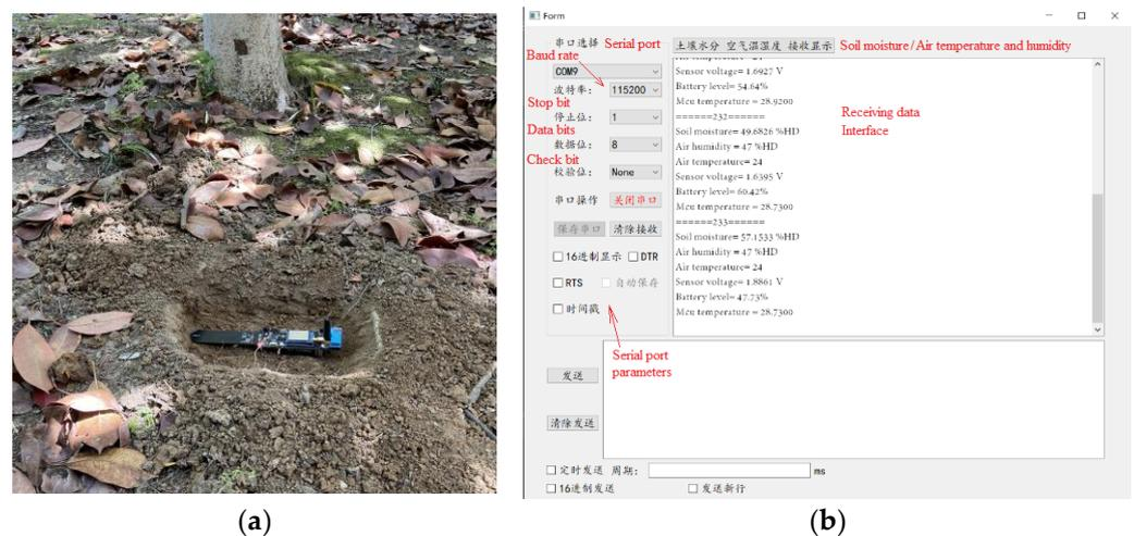
**Figure 6.** Field data acquisition: (a) field testing of a soil wireless sensor node; (b) data-receiving interface on a PC terminal.
