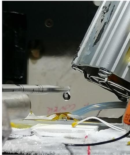
**Figure 3.** Example of drop injection (side view).
