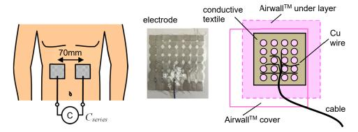
Figure 2. Typical electrodes attached to the skin; conductive textiles are used.
