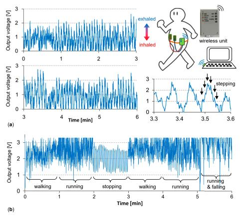
**Figure 5.** Abdomen capacitance signals measured by the wireless unit (**a**) during gentle walking and (**b**) during harder walking for 6 min.
