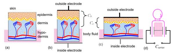
**Figure 1.** (a) Skin structure. Model of the electrodes constructing the capacitance across the skin under (b) exhalation and (c) inhalation conditions. (d) The two capacitances are considered to connect in series inside the body and are measured by the outside circuit.
