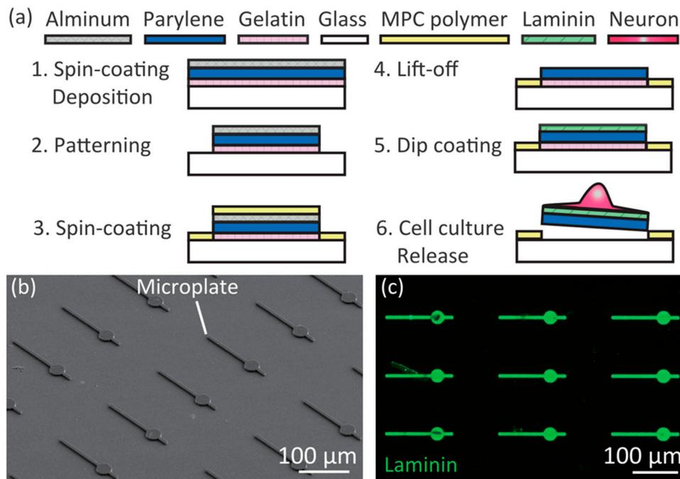
**Figure 2.** Fabrication of the microplate device. (a) Fabrication process; (b) Scanning electron microscopy (SEM) image of fabricated microplates on glass; (c) Immunostained image of laminin (green) on the microplates.
