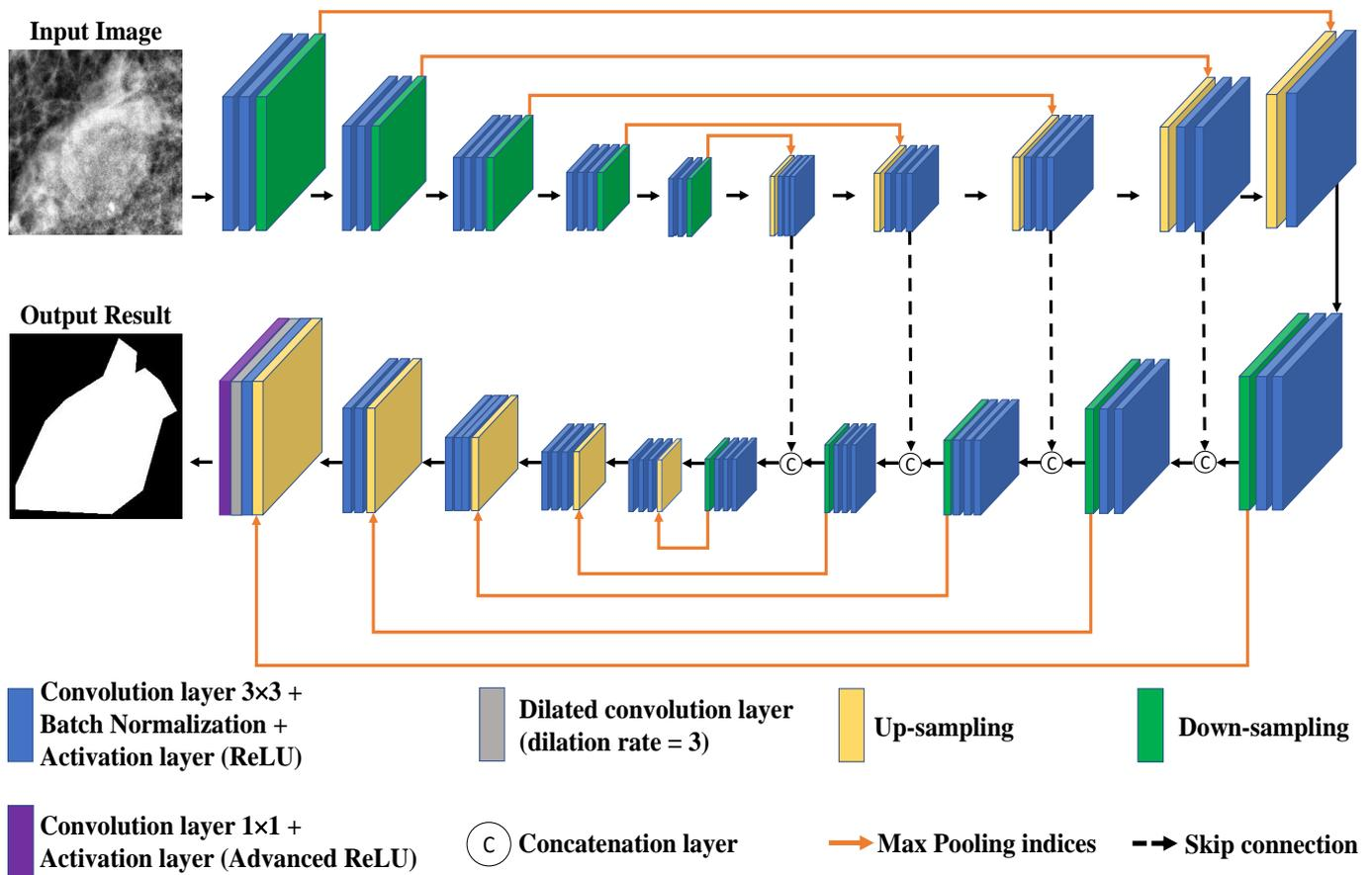
Figure 4. Architecture of the proposed Connected-SegNets model.
