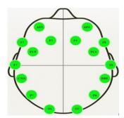
Figure 3. Electrode Placement Channel Electroencephalography (EEG) Headset.
