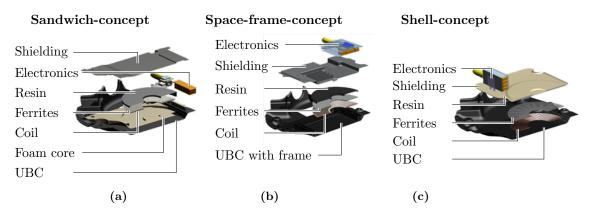
**Figure 6.** Proposed concepts of functionally integrated CPMs: (a) sandwich concept; (b) space-frame concept; and (c) shell concept.
