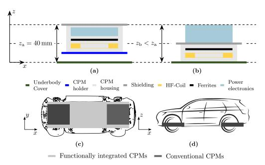
**Figure 4.** Qualitative comparison of the z-dimension of: (**a**) conventional designs of CPMs with a maximum transmission power of 3.6 kW given in [12]; (**b**) the functionally integrated CPM to be developed with a transmission power of more than 3.6 kW; and (**c**,**d**) possible installation space of CPM designs in (**c**) xy-plane and (**d**) xz-plane.
