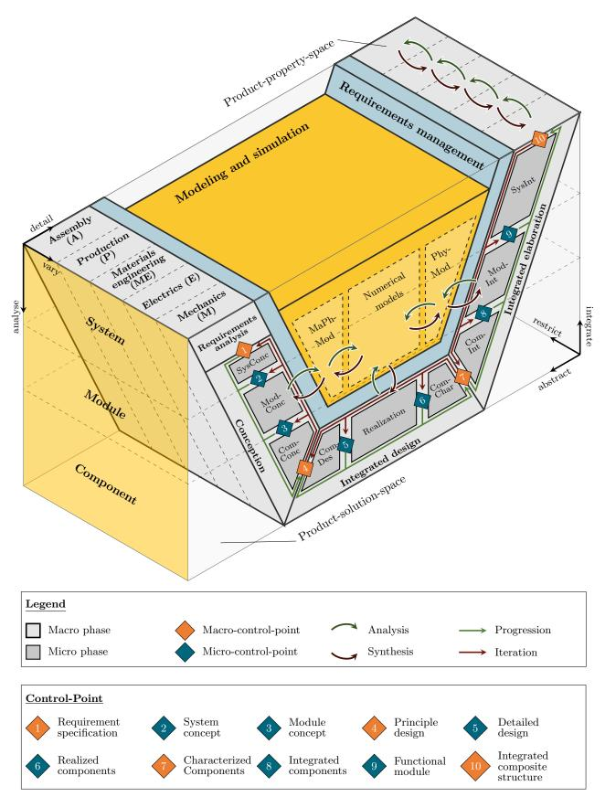
**Figure 2.** Systematic design approach to the development of functionally integrated mechanical-electrical lightweight systems.
