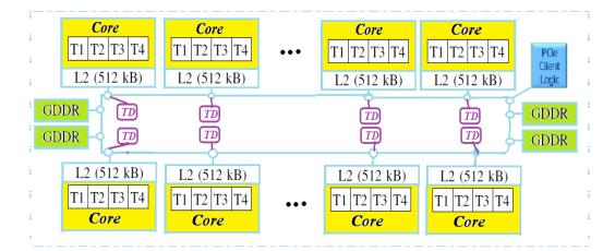
Figure 1. Intel Xeon Phi Architecture.
