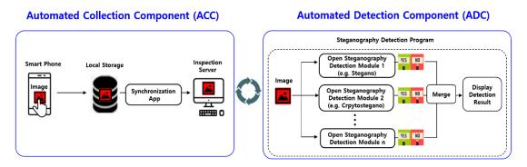
Figure 4. Design of our proposed system with two main components (automated collection component and automated detection component).
