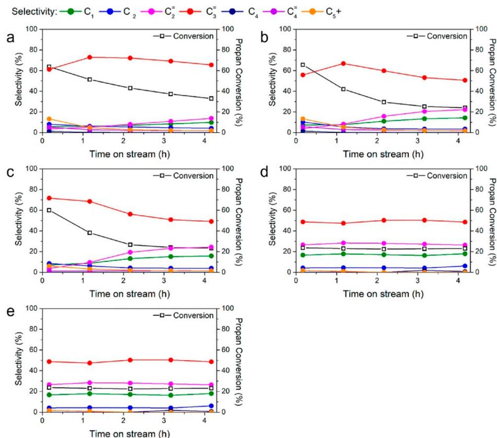
**Figure 8.** Catalytic performance of PDH over supported Pt-Sn catalysts at 620 °C: (a) Pt-Sn/Beta(300), (b) Pt-Sn/Beta(38), (c) Pt-Sn/ $\theta$ -Al<sub>2</sub>O<sub>3</sub>, (d) Pt-Sn/Q6, and (e) blank test in the absence of catalysts.
