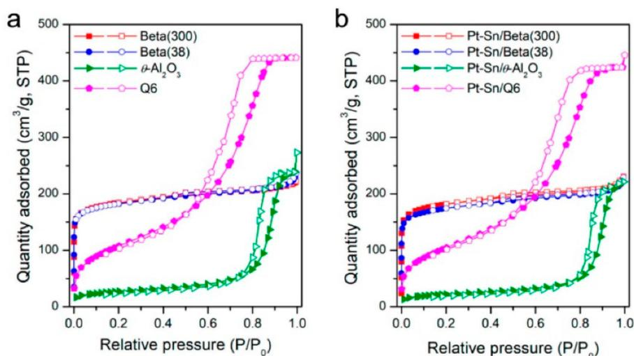
Figure 1. N<sub>2</sub> adsorption–desorption isotherms of (a) supports and (b) supported Pt-Sn catalysts.
