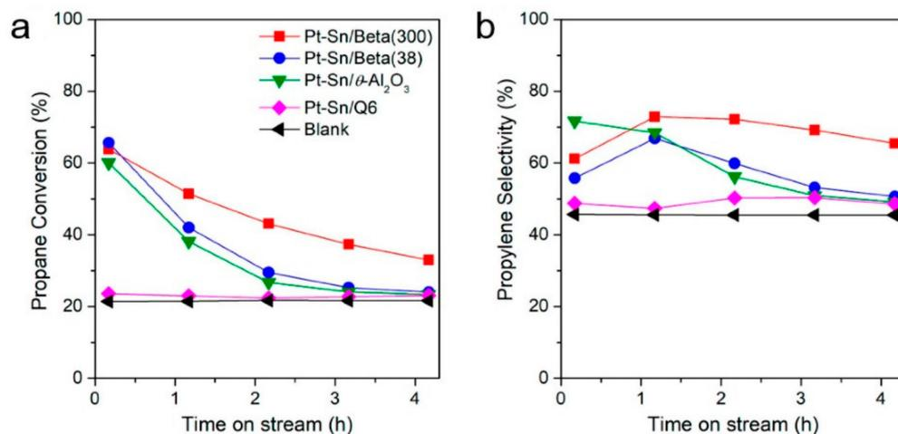
**Figure 7.** Catalytic performances over different supported Pt-Sn catalysts in propane dehydrogenation (PDH) at 620 °C: (a) propane conversion (%) and (b) propylene selectivity (%).
