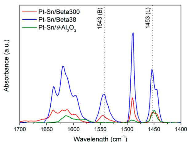
Figure 3. FT-IR spectra of adsorbed pyridine over supported Pt-Sn catalysts.
