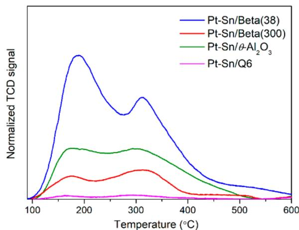
Figure 2. NH<sub>3</sub>-TPD profiles of supported Pt-Sn catalysts.
