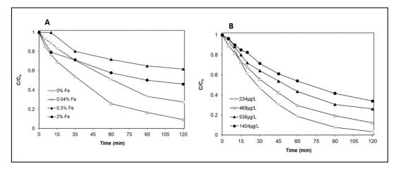
**Figure 14.** (A) Signifies the effect of iron doping level, where 0.5% Fe/TiO<sub>2</sub> showed the most efficient photocatalytic degradation. (B) represents the effect of initial SMZ concertation; as noted, there is a decrement in the rate constant as the concentration of SMZ increases. Adapted with permission from [123]. Copyright 2019 Elsevier.
