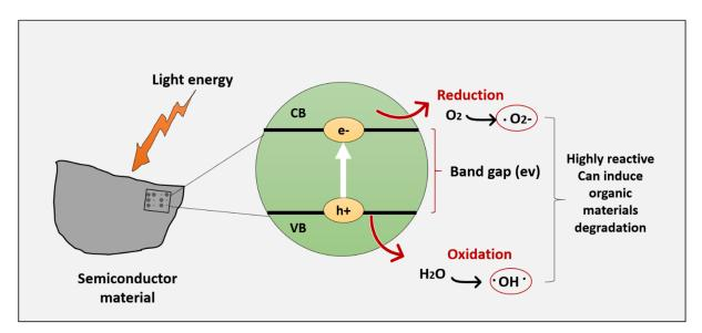
Figure 2. General photocatalytic mechanism. Adapted from [38] with modifications.
