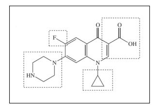
Figure 5. Different attack sites in CIP structure by free radicals generated by photocatalytic reaction.
