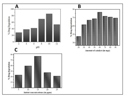
**Figure 9.** Different parameters were applied to degrade the antibiotic norfloxacin using Mn:ZnS Quantum Dots. (**A**) showing the effect of pH on norfloxacin, with pH = 10 owining the best photocatalytic efficiency(**B**) represents a bar chart with the effect of the number of catalysts used. (**C**) signifies the effect of the initial antibiotic concentration. Adapted from [100].
