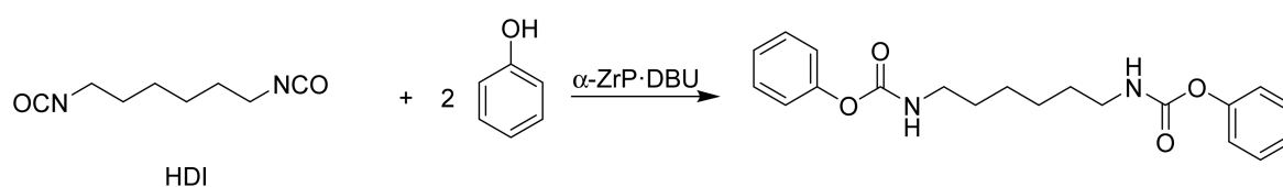
Scheme 1. Reaction of HDI and phenol with \alpha -ZrP DBUs.
