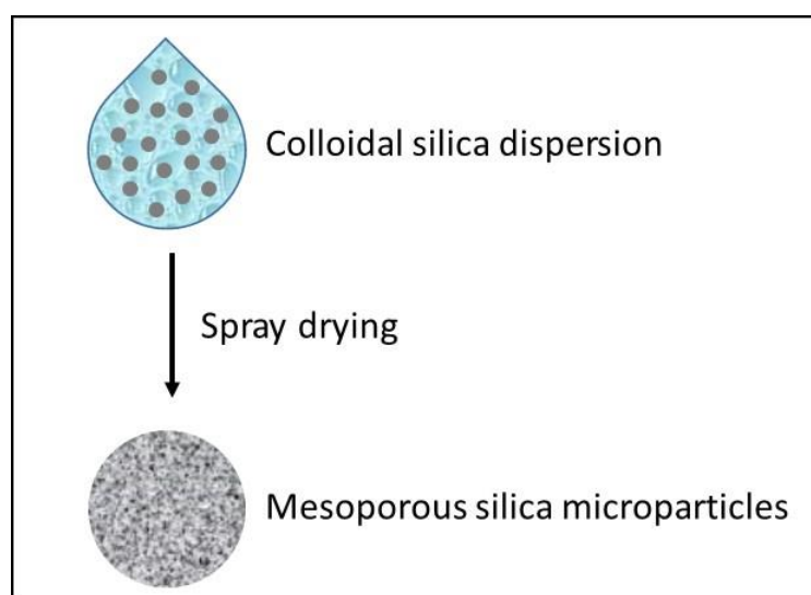
Figure 5. Spray-drying of a colloidal silica dispersion.
