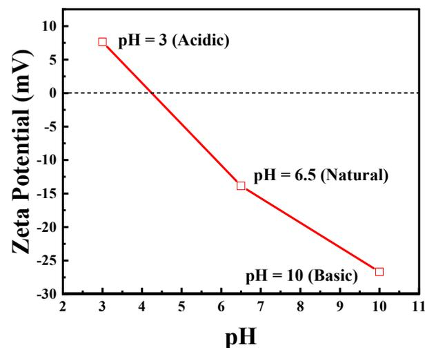
Figure 4. Zeta potential at different pH of the synthesized exfoliated g-C<sub>3</sub>N<sub>4</sub>. Reproduced with permission from [18].
