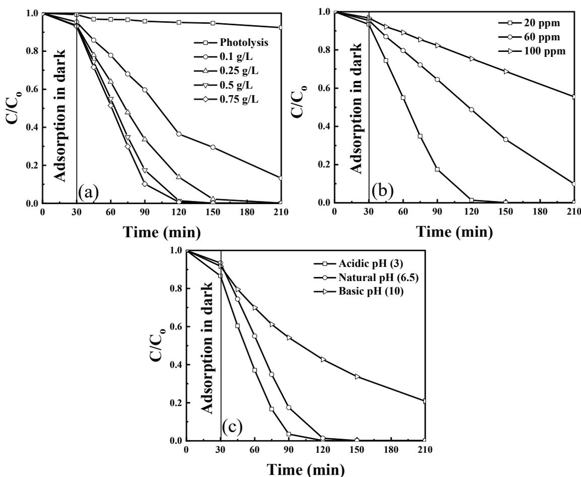
**Figure 5.** Phenol degradation at preselected (a) catalyst concentration (at 20 ppm and natural pH) (b) pollutant concentration (at 0.5 g/L and natural pH), and (c) pH of the solution (at 0.5 g/L and 20 ppm); airflow = 50 mL/min. Reproduced with permission from [18].
