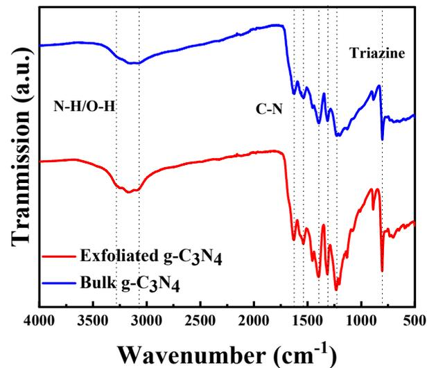
Figure 3. Fourier transform infrared spectra of bulk and exfoliated g-C<sub>3</sub>N<sub>4</sub>.
