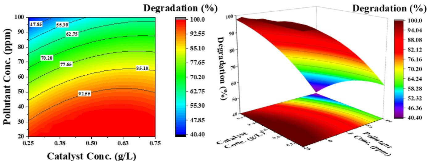
Figure 9. Effect of catalyst concentration and pollutant concentration on the degradation of phenol: pH was kept constant at 6.5.
