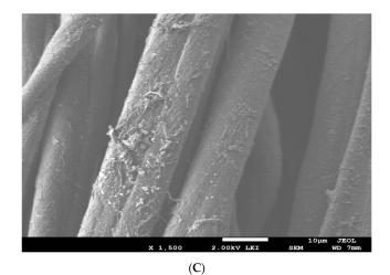
Figure 2. SEM images of CF (A), 6 mL sample AgNp-CF (B), catalase immobilized onto B sample (C).
