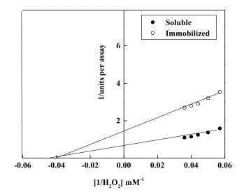
**Figure 7.** Lineweaver-Burk plot relating soluble catalase and immobilized catalase reaction velocity to  $H_2O_2$  concentrations.
