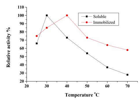
**Figure 5.** Optimum temperature of soluble catalase and immobilized catalase. Each point represents the average of two experiments.
