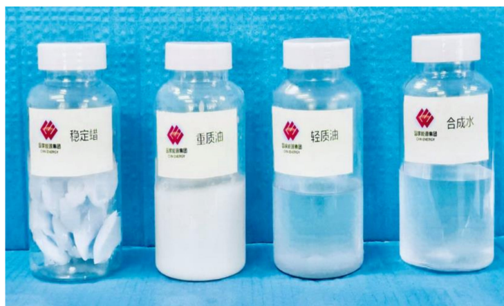
Figure 16. FTS products acquired at a million-ton FTS plant using the CNFT-1 catalyst. From left to right are the stable wax, heavy oil, light oil, and synthetic water, respectively.
