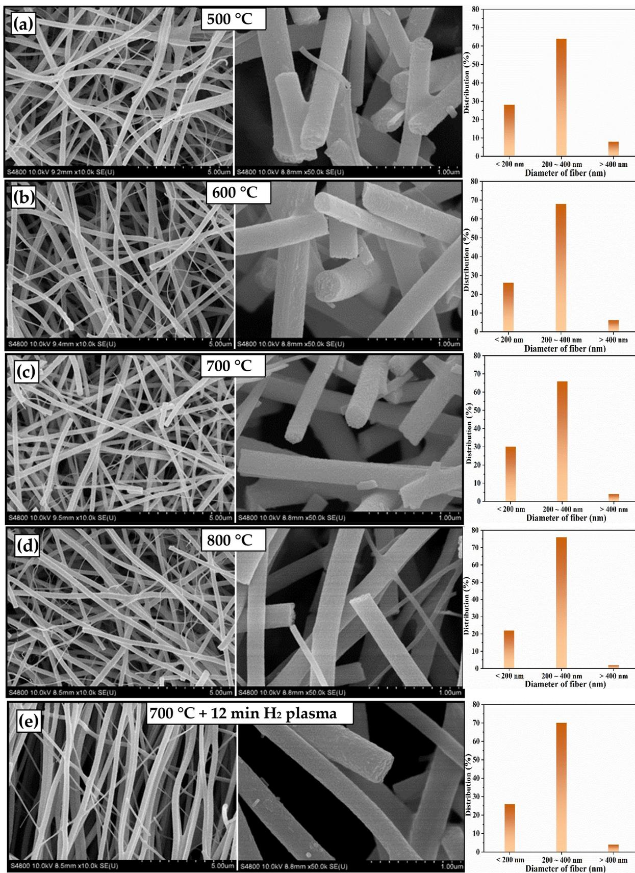
Figure 1. SEM images of TiO<sub>2</sub> fibers obtained after calcination at different temperatures and plasma treatments: (a) TiO<sub>2</sub>-500 °C, (b) TiO<sub>2</sub>-600 °C, (c) TiO<sub>2</sub>-700 °C, (d) TiO<sub>2</sub>-800 °C, and (e) TiO<sub>2</sub>-PH72.
