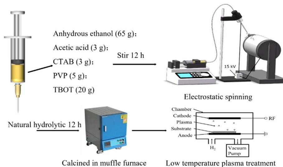
**Figure 13.** Process flow chart of electrospinning TiO<sub>2</sub> fiber preparation; heat treatment and plasma modification.
