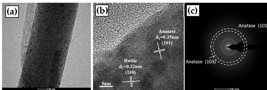
Figure 3. TEM observation of the TiO<sub>2</sub> fiber annealed at 700 °C; (a) TEM image of local magnification; (b) HRTEM image and lattice annotation of anatase and rutile, and (c) calibration of diffraction pattern.
