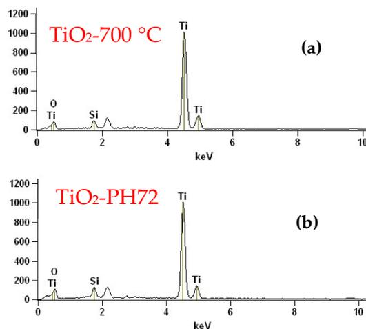
Figure 7. EDX images of the (a) TiO<sub>2</sub>-700 °C and (b) TiO<sub>2</sub>-PH72 samples.
