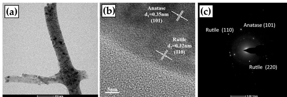
Figure 4. TEM observation of the TiO<sub>2</sub> fiber annealed at 800 °C; (a) TEM image of local magnification; (b) HRTEM image and lattice annotation of anatase and rutile, and (c) calibration of diffraction pattern.
