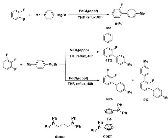
**Scheme 10.** Cross-coupling of fluoro-aromatic with Grignard reagents.
