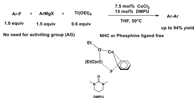
**Scheme 20.** Cobalt-catalyzed C–F bond activation and Co–Ti co-oxidative addition reaction transition state.
