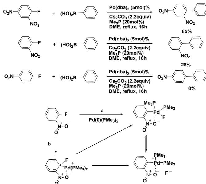
**Scheme 7.** Palladium-catalyzed C–F bond activation of nitrofluoro-aromatics and the reaction mechanism.
