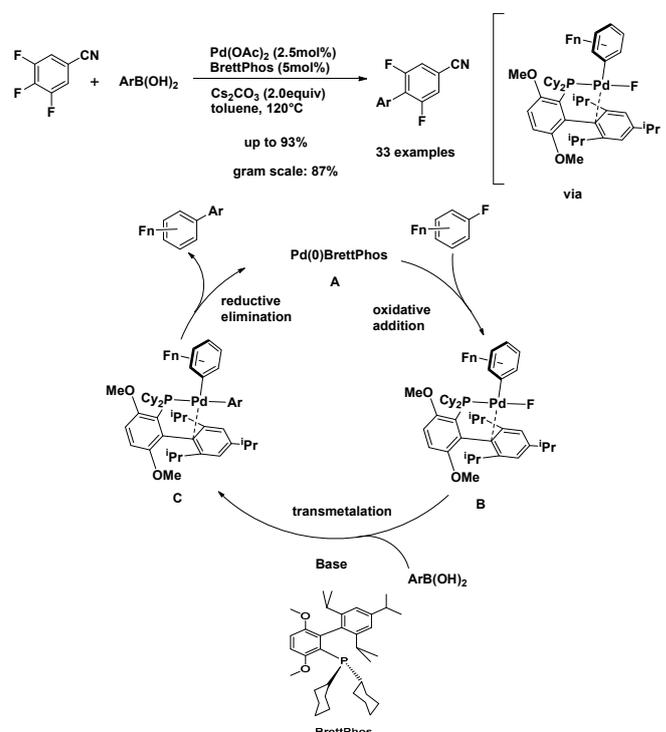
**Scheme 15.** Pd(OAc)<sub>2</sub>/BrettPhos-catalyzed C–F bond activation of multifluoro-aromatics and plausible reaction pathway.
