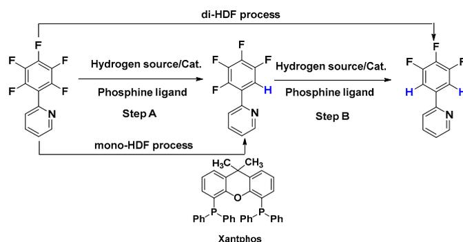
**Scheme 19.** Rh-catalyzed HDF of heterocyclic substituted multifluoro-aromatics and selectivity pathways for phosphine ligand control.
