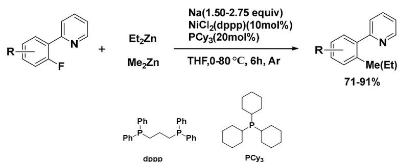
**Scheme 2.** NiCl<sub>2</sub> (dppp) catalyzed cross-coupling of fluoro-aromatics with organozinc reagents.
