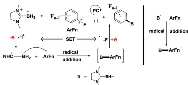
**Scheme 34.** Photocatalytic defluoro-boration of multifluoro-aromatics with NHC borane.
