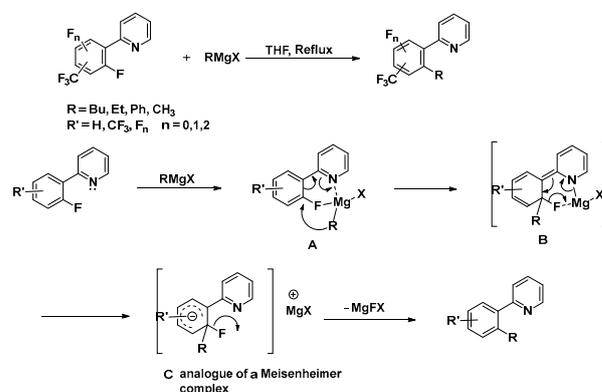
**Scheme 26.** The cross-coupling of multifluoro-arenes with Grignard reagents via pyridine-directed cleavage of the C–F bond in the absence of transition metal.
