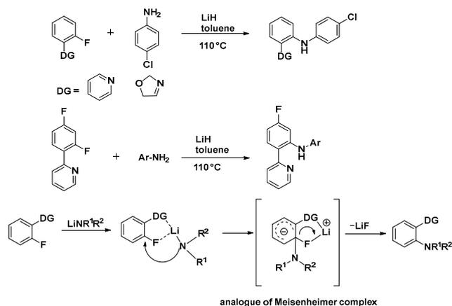
**Scheme 28.** Cross-coupling of fluoro-aromatics with amines under transition metal-free conditions.
