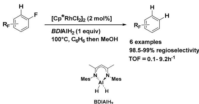
**Scheme 18.** Rh-catalyzed HDF of multifluoro-aromatics (BDIAIH<sub>2</sub>, hydrocarbon-soluble aluminum dihydride).
