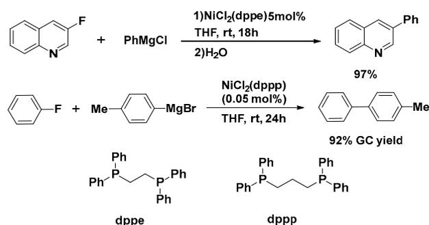
**Scheme 1.** Activation of C–F Bond catalyzed by nickel complexes with bidentate phosphine ligand.
