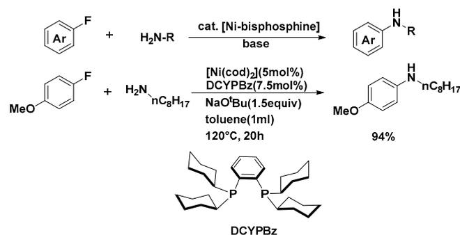
**Scheme 5.** Nickel-catalyzed amination of fluoro-aromatics with primary amines.
