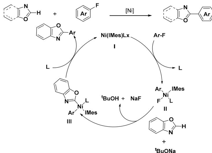
**Scheme 6.** Nickel-catalyzed cross-coupling of fluoro-aromatics with oxazole and the mechanistic pathway.
