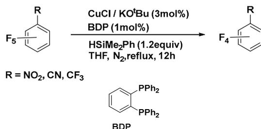
**Scheme 17.** Cu-catalyzed HDF of pentafluoroaromatics.
