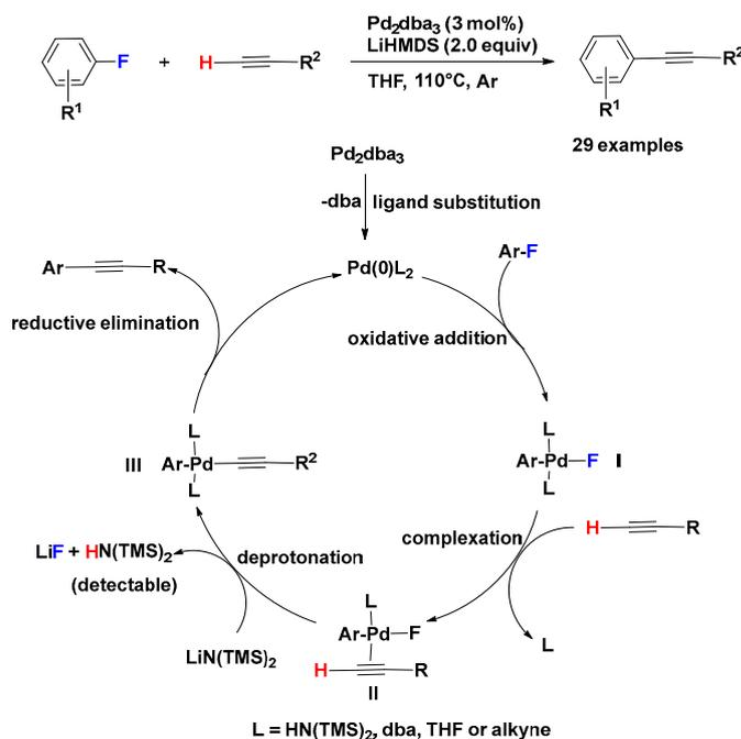
**Scheme 13.** Plausible mechanism of LiHMDS-promoted Sonogashira cross-coupling of fluoro-aromatics with terminal alkynes catalyzed with palladium.
