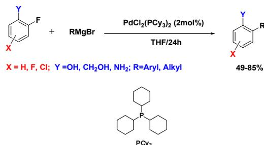
**Scheme 11.** Cross-coupling of fluoro-aromatics with Grignard reagent catalyzed by  $\text{PdCl}_2(\text{PCy}_3)_2$ .
