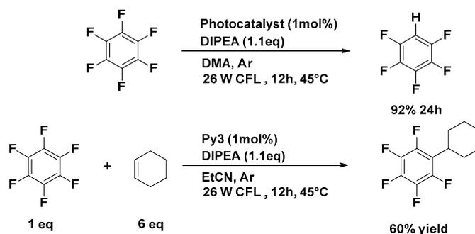
**Scheme 33.** Photocatalytic HDF of perfluorobenzene and cross-coupling of multifluorobenzene with olefinic substrate.
