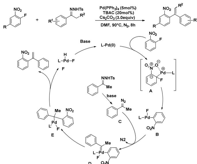
**Scheme 8.** Pd-catalyzed cross-coupling of electron-deficient fluoro-aromatics with N-tosylhydrazones and the reaction pathway.
