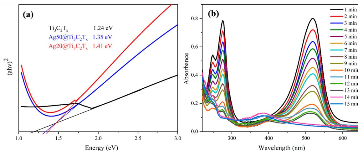
**Figure 5.** (a) Band gap of  $\text{Ti}_3\text{C}_2\text{T}_x$ ,  $\text{Ag20@Ti}_3\text{C}_2\text{T}_x$ ,  $\text{Ag50@Ti}_3\text{C}_2\text{T}_x$ ; (b) photocatalytic degradation of safranin dye using 5 mg of  $\text{Ag50@Ti}_3\text{C}_2\text{T}_x$  catalyst at different time intervals.
