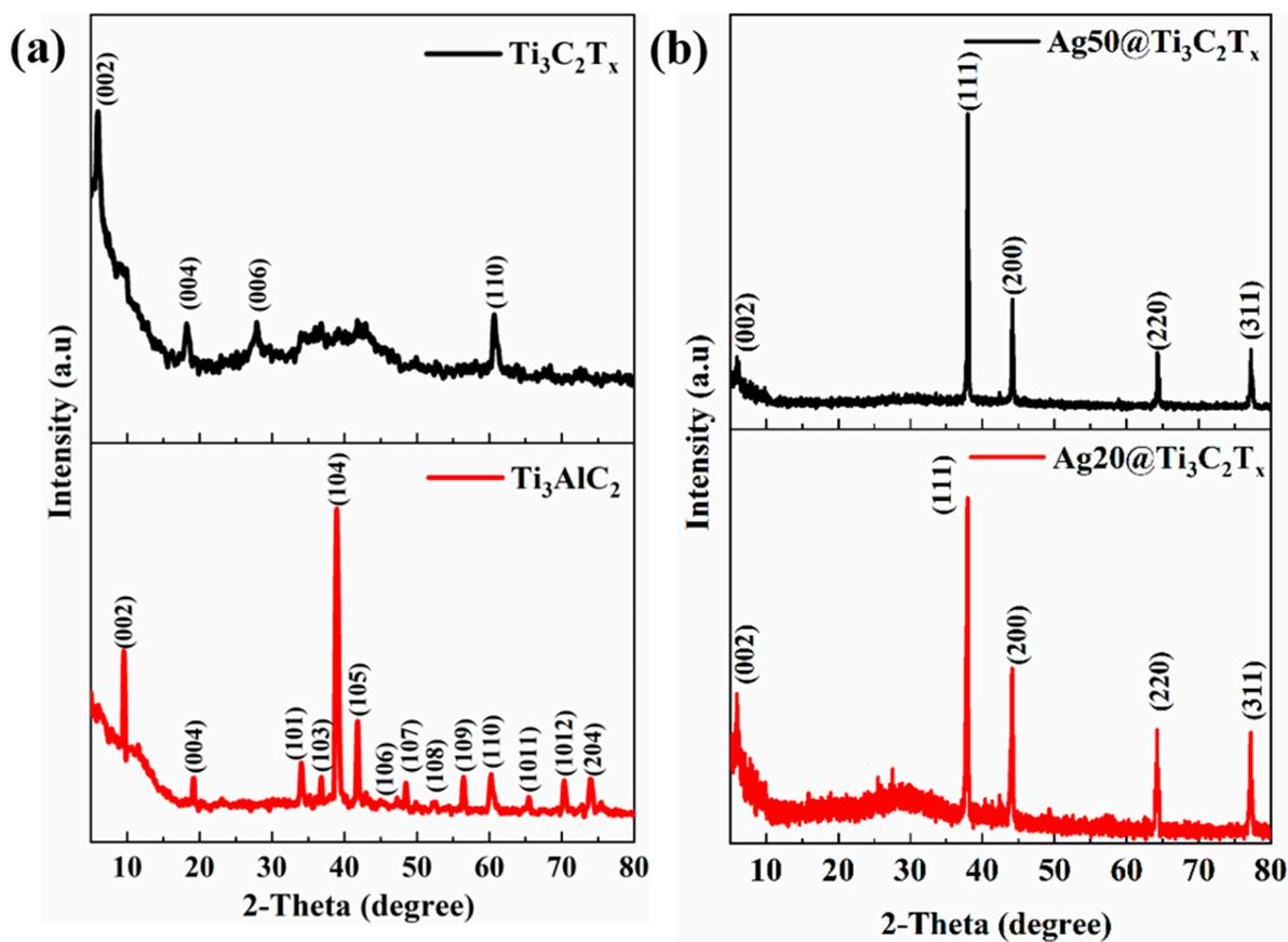
Figure 1. XRD analysis of (a)  $\text{Ti}_3\text{AlC}_2$ ,  $\text{Ti}_3\text{C}_2\text{T}_x$  and (b)  $\text{Ag}_{20}@\text{Ti}_3\text{C}_2\text{T}_x$ ,  $\text{Ag}_{50}@\text{Ti}_3\text{C}_2\text{T}_x$ .
