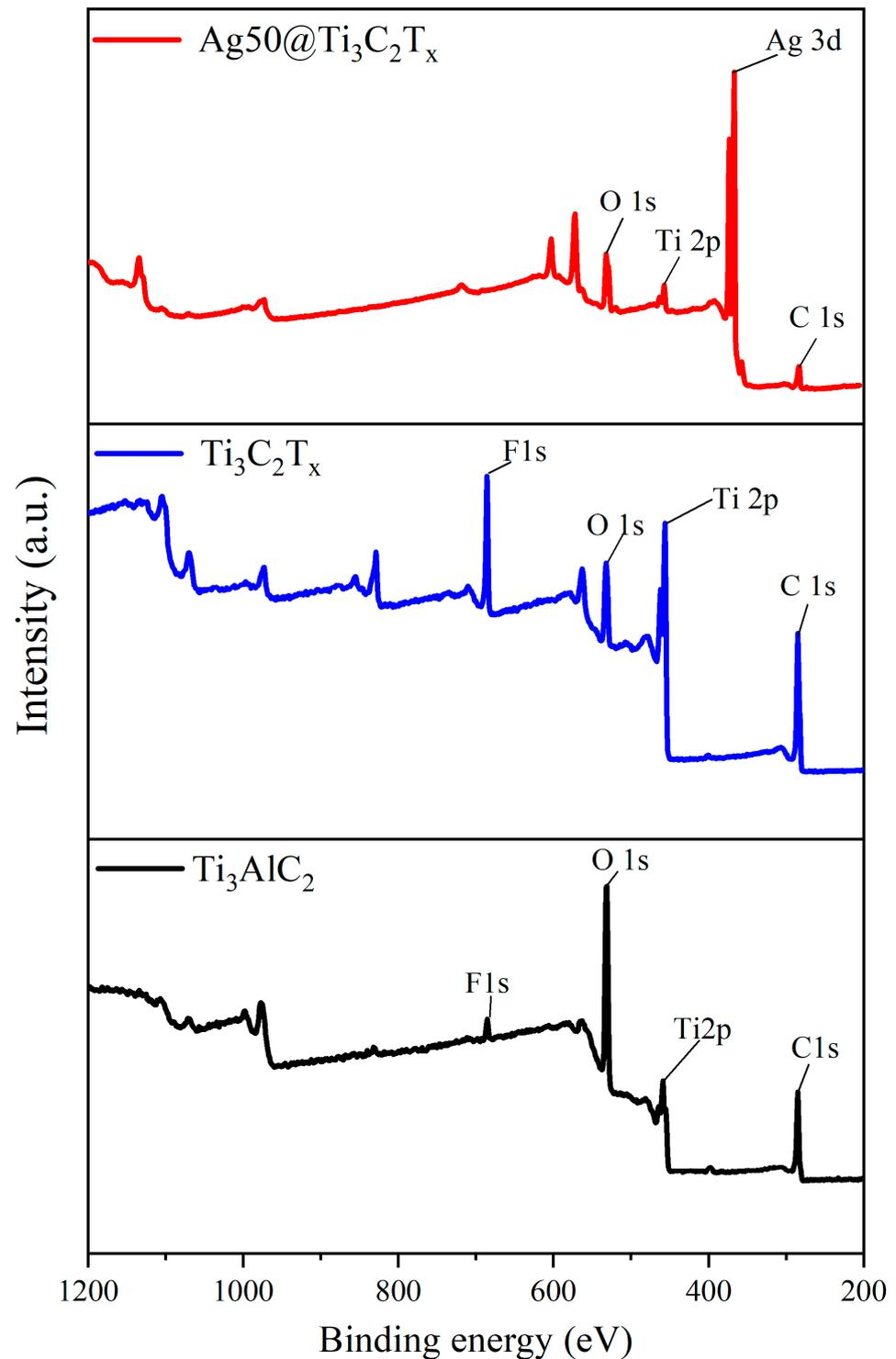
**Figure 2.** XPS Survey of Ti<sub>3</sub>AlC<sub>2</sub>, Ti<sub>3</sub>C<sub>2</sub>T<sub>x</sub>, Ag50@Ti<sub>3</sub>C<sub>2</sub>T<sub>x</sub>.
