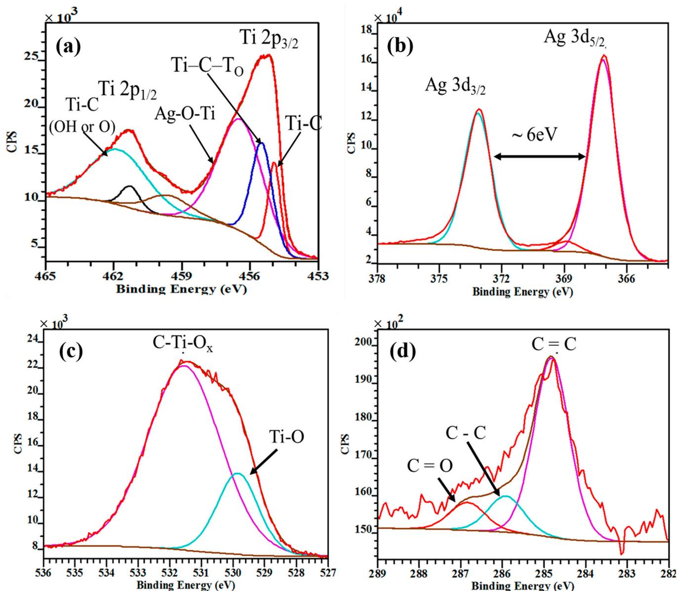
**Figure 3.** XPS analysis of silver-doped MXene (a) Ti 2p (b) Ag 3d (c) O 1s (d) C 1s.
