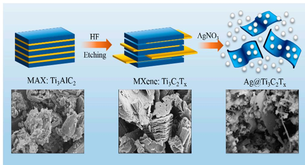
**Figure 8.** Schematic representation for the synthesis of  $\text{Ag@Ti}_3\text{C}_2\text{T}_x$ .
