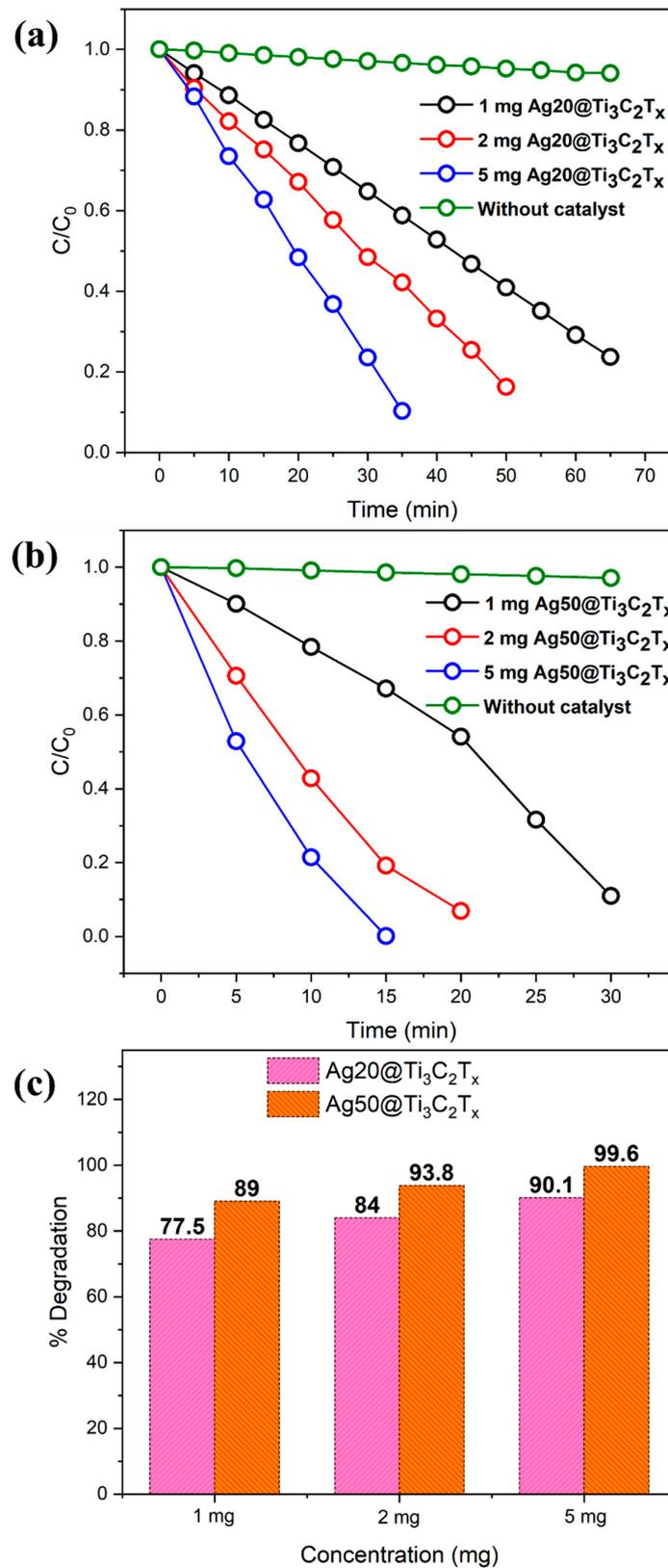
**Figure 6.** (a) Photocatalytic activity of Ag20@Ti<sub>3</sub>C<sub>2</sub>T<sub>x</sub> and (b) Ag50@Ti<sub>3</sub>C<sub>2</sub>T<sub>x</sub>; (c) percentage degradation efficiency of prepared catalysts.
