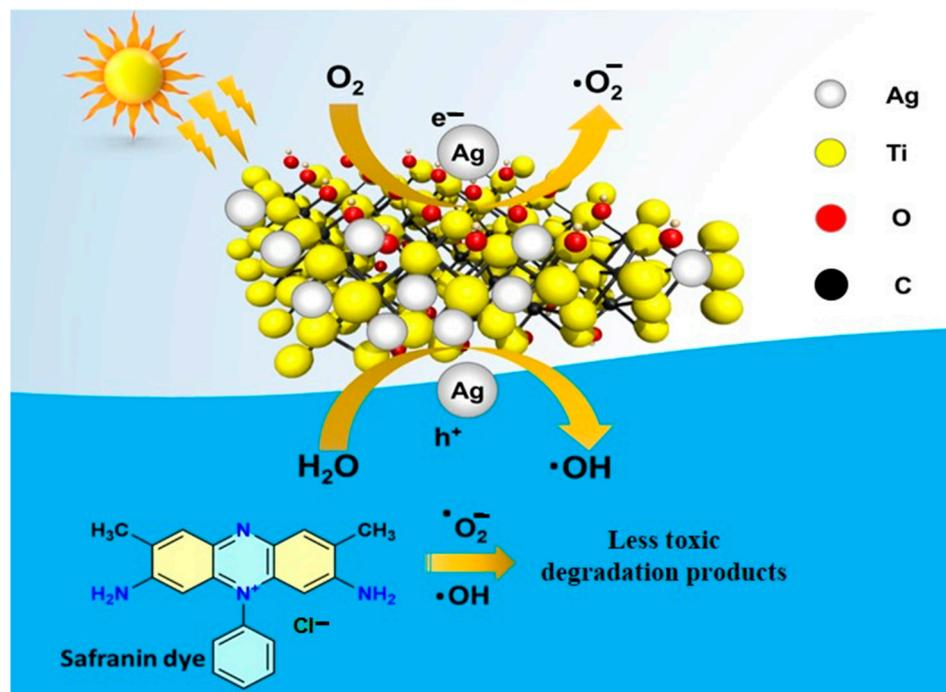
**Figure 7.** Proposed photocatalytic mechanism for the degradation of safranin dye using  $\text{Ag}@\text{Ti}_3\text{C}_2\text{T}_x$  nanocomposite.
