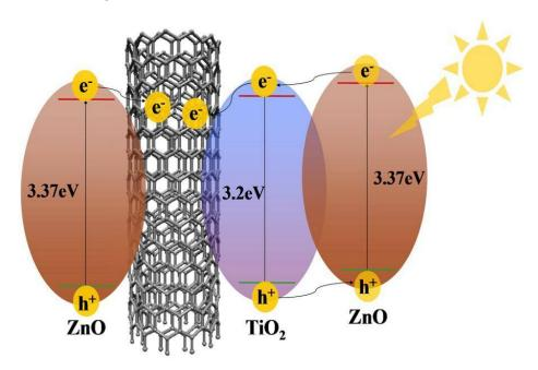
Figure 4. Schematic electron-hole separation process of CNT/TiO<sub>2</sub>/ZnO composites.
