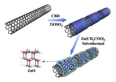
Figure 1. Schematic illustration of the ternary carbon nanotubes (CNTs)/TiO<sub>2</sub>/ZnO composites.
