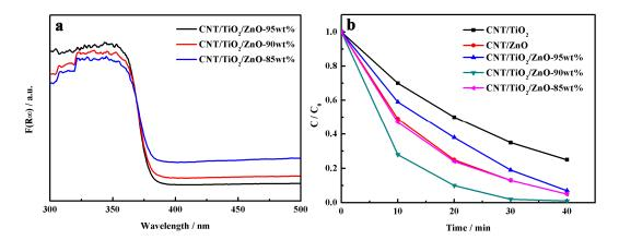
**Figure 3.** (a) UV-vis diffuse reflectance spectroscopy (DRS) patterns of CNT/TiO<sub>2</sub>/ZnO-95 wt %, CNT/TiO<sub>2</sub>/ZnO-90 wt % and CNT/TiO<sub>2</sub>/ZnO-85 wt %; (b) change of concentration of rhodamine B (RhB) during degradation process in UV-vis light irradiation of CNT/TiO<sub>2</sub>, CNT/ZnO, CNT/TiO<sub>2</sub>/ZnO-95 wt %, CNT/TiO<sub>2</sub>/ZnO-90 wt % and CNT/TiO<sub>2</sub>/ZnO-85 wt %.
