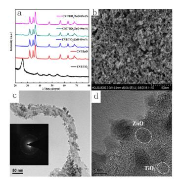
**Figure 2.** (a) X-ray powder diffraction (XRD) patterns of CNT/TiO<sub>2</sub>, CNT/ZnO, CNT/TiO<sub>2</sub>/ZnO-95 wt %, CNT/TiO<sub>2</sub>/ZnO-90 wt % and CNT/TiO<sub>2</sub>/ZnO-85 wt %; (b) SEM image of CNT/TiO<sub>2</sub>/ZnO-90 wt %; (c) Transmission electron microscopy (TEM) image with SAED pattern (inset) of CNT/TiO<sub>2</sub>/ZnO-90 wt %; (d) HRTEM image of CNT/TiO<sub>2</sub>/ZnO-90 wt %.
