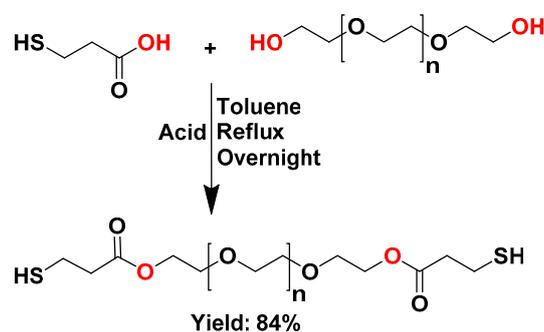
Figure 1. Synthesis of poly(ethylene glycol) (PEG)-dithiol [22].
