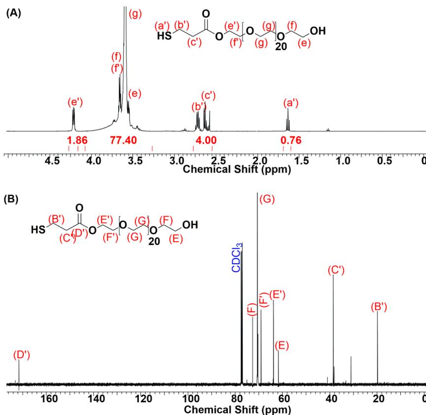
**Figure 6.** (A) <sup>1</sup>H-NMR and (B) <sup>13</sup>C-NMR of PEG<sub>1000</sub>-monothiol [<sup>1</sup>H-NMR (500 MHz, CDCl<sub>3</sub>):  $\delta$  4.21 (2H) 3.61(86H) 2.72 (2H) 2.63 (2H) 1.65 (1H); <sup>13</sup>CNMR (500 MHz, CDCl<sub>3</sub>):  $\delta$  171.5, 72.66, 70.6, 69.1, 63.8, 61.72, 38.5, 19.7].
