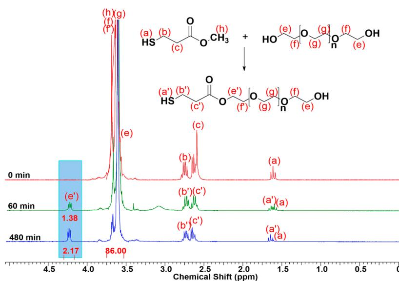
**Figure 5.**  $^1\text{H}$ -NMR monitoring of the kinetics of transesterification of MP-SH with PEG<sub>1000</sub> [480 min:  $^1\text{H}$ -NMR (500 MHz,  $\text{CDCl}_3$ ):  $\delta$  4.23 (2H) 3.61(86H)].
