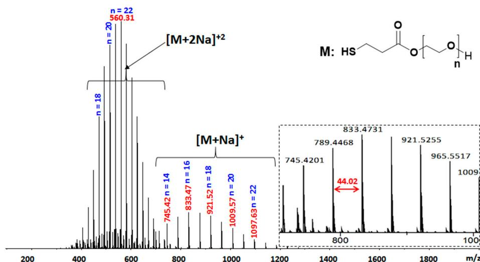
**Figure 7.** MALDI-ToF mass spectra of PEG<sub>1000</sub> monothiol. Inset: The zoomed version of the 14- to 20-mer fractions, 44 m/z = PEG repeat unit.
