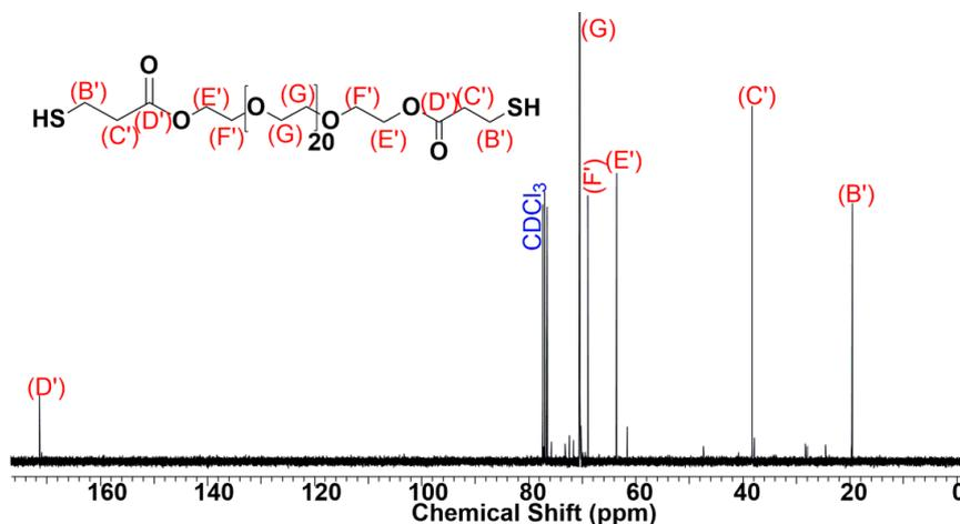
**Figure 8.** <sup>13</sup>C-NMR of PEG<sub>1000</sub> dithiol [<sup>13</sup>C-NMR (500 MHz, CDCl<sub>3</sub>):  $\delta$  171.3, 70.4, 68.9, 63.6, 38.3, 19.6].
