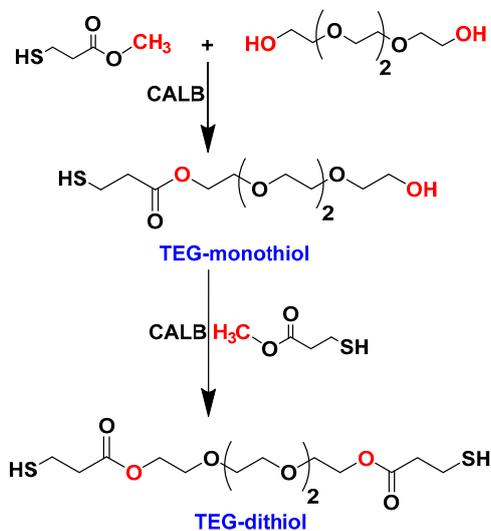
**Figure 3.** CALB-catalyzed transesterification of MP-SH with TEG.
