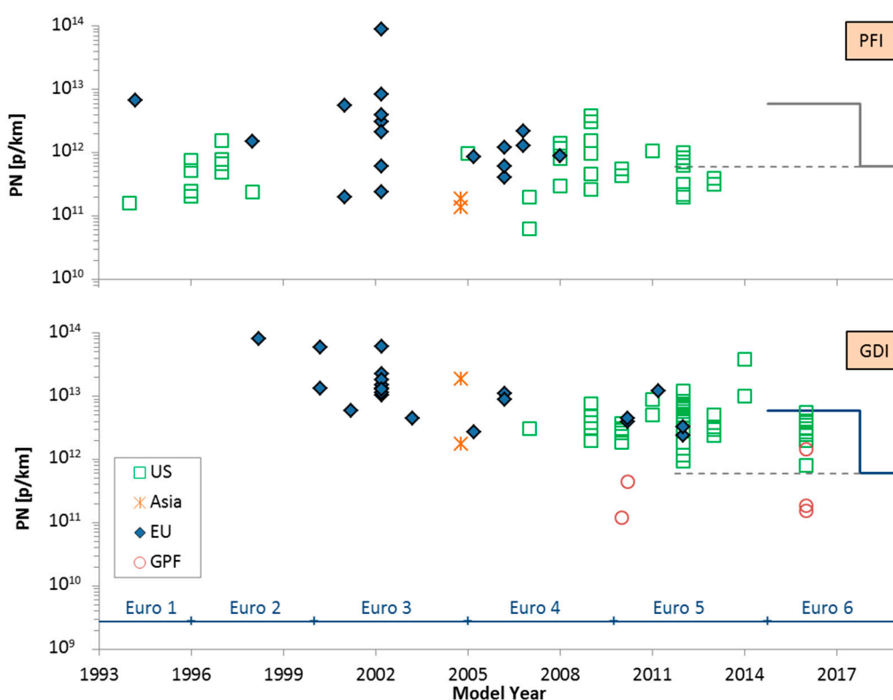
Figure A1. Total particle number (PN) emissions for gasoline direct injection (GDI) (lower panel) and port fuel injection (PFI) (upper panel) vehicles. Dashed line shows solid PN (SPN) limit for diesel vehicles (only EU). Solid line shows SPN limits for GDI vehicles (only EU).
